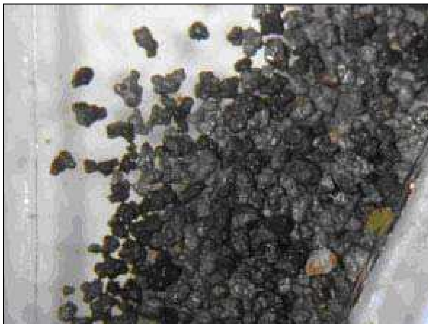
Figure 5.83. Lead grains found in sand-glasses.
