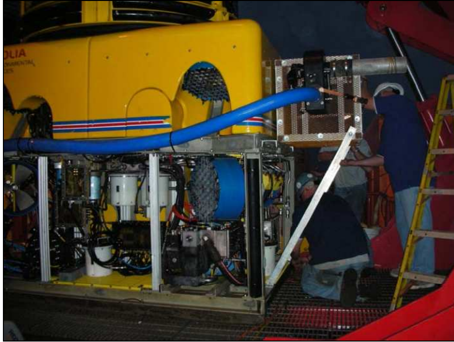
Figure 3.2. Excavation dredge pump and screening system.
