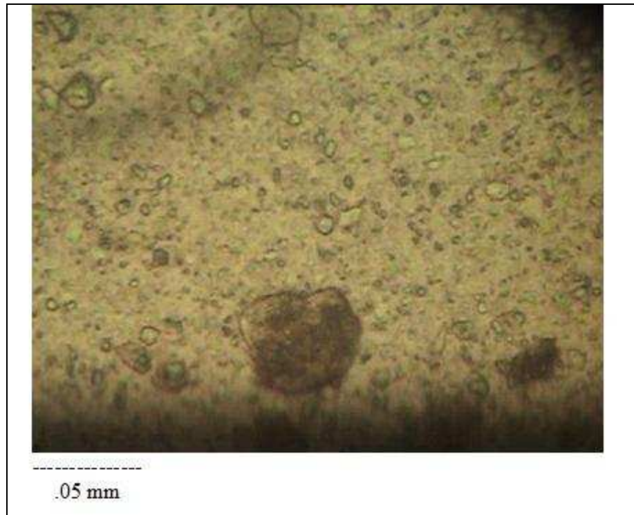
Figure 2.5. The fine fraction (less than 0.063mm) of core 2, illustrating the silt-sized quartz in the core.
