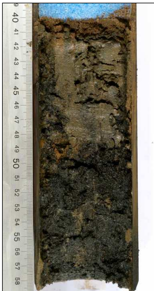
Figure 2.9. Core 1, illustrating the oxidized portion of the core.
