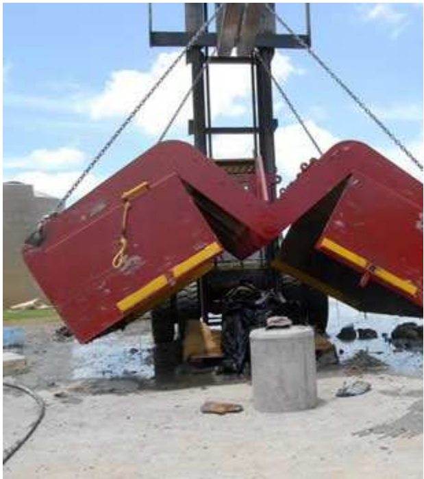
Here, the open LART reveals its "clamshell" construction, and a forklift is maneuvered into place behind the encrustation. To prevent the
