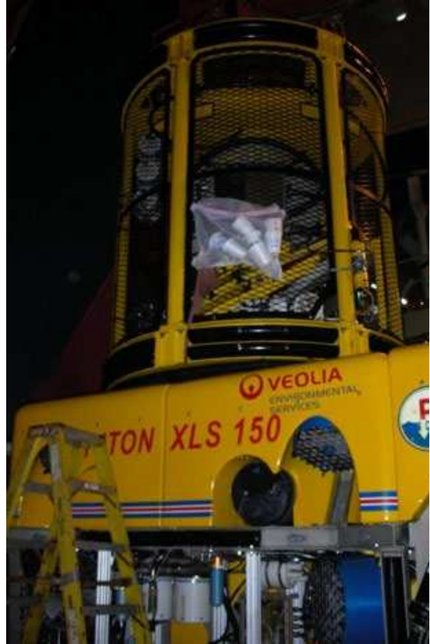
The ROV which was used to investigate the shipwreck site, a Perry Triton XLS-17 provided by Veolia Environmental, is seen at right. The primary tools for artifact recovery were suction pickers, commonly called "sticky feet." Also visible in the picture is a bag of styrofoam cups, which were crushed by the water pressure at the deep site.
