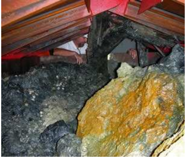
Above, the stern encrustation is seen within the LART that was used to transport the encrustation to the Conservation Research Laboratory at Texas A&M; University.
