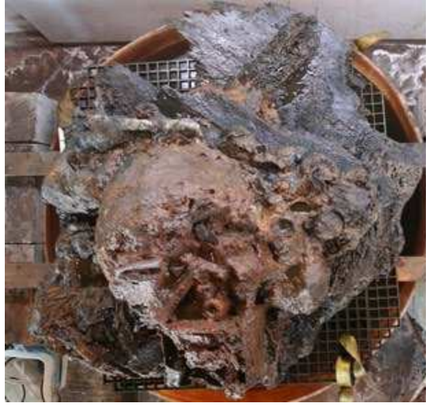
The stern encrustation is seen from above here, as it is prepared to be lowered into the vat where it will undergo desalination and further treatment.
