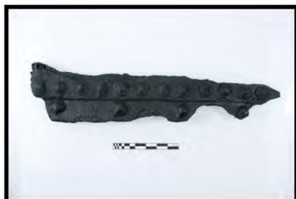
FIGURE 126. RIVETED PLATE FROM STEAM DRUM (ARTIFACT NP-50; SCALE INCHES)
