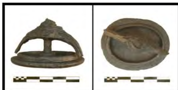
FIGURE 141. LARGER SIZED HAND HOLE CLEANING COVER (ARTIFACT 120-053; SCALE CM)
