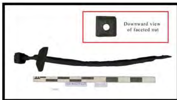
FIGURE 109. TYPE 1 MASSIVE BOLT AND WASHER FASTENER FOR CYLINDER BASE/BED FRAME TIMBERS (ARTIFACT 138-003; SCALE CM/DM)
