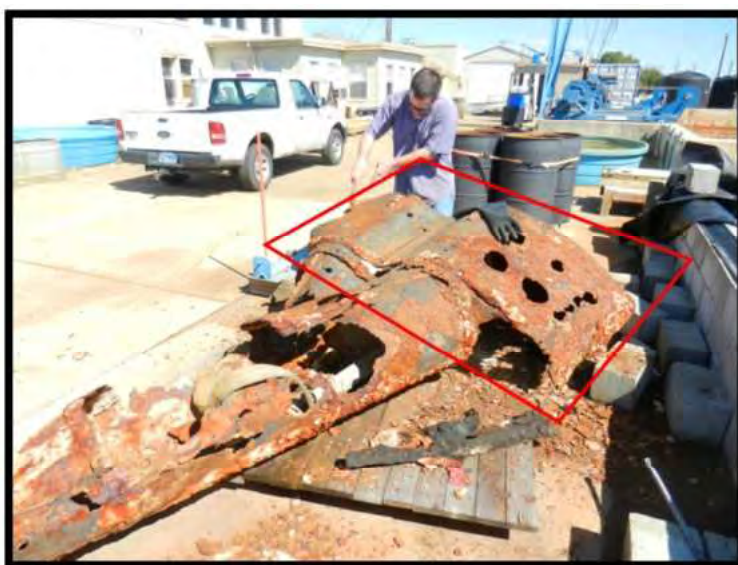
FIGURE 190. REMAINS OF LOWER COMBUSTION CHAMBER (ARTIFACT IS UPSIDE DOWN)
