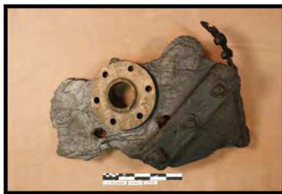
FIGURE 181. REAR FIREBOX FEED WATER PIPE (ARTIFACT 133-007; SCALE CM/DM)
