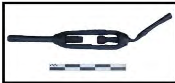
FIGURE 114. LARGE TURN BUCKLE FROM A-FRAME (ARTIFACT 117-002; SCALE CM/DM)
