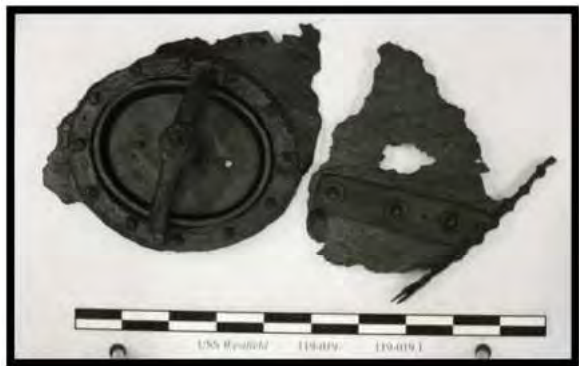
FIGURE 143. MAN HOLE ACCESS HATCH FROM REAR BOILER BARREL (ARTIFACT 119-019; SCALE DM)
