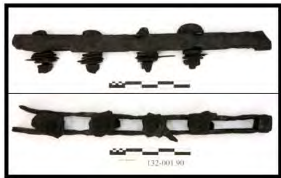
FIGURE 195. GIRDER STAY FROM TOP OF COMBUSTION CHAMBER (ARTIFACT 132-001.90; SCALE CM)
