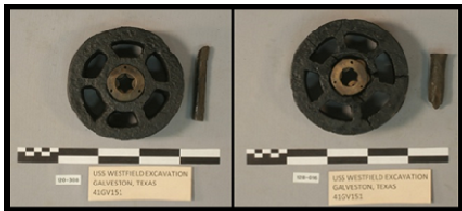
FIGURE 203. CAST IRON SHEAVES WITH BRASS BEARINGS (ARTIFACTS 120-308 AND 128-016)
