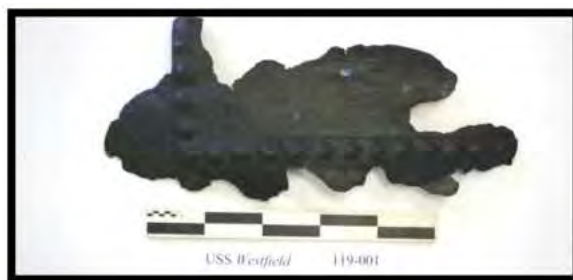
FIGURE 173. SMALL SECTION OF PLATING FROM OUTER BOILER BARREL (ARTIFACT 119-001; SCALE CM/DM)
