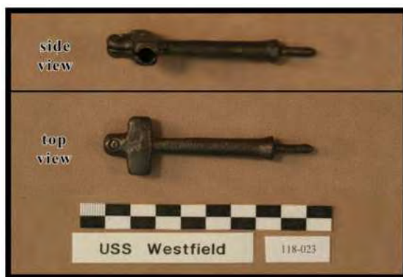
FIGURE 286. BRASS SOCKET TRAMMEL FROM NAVIGATIONAL BEAM COMPASS (ARTIFACT 118-023)
