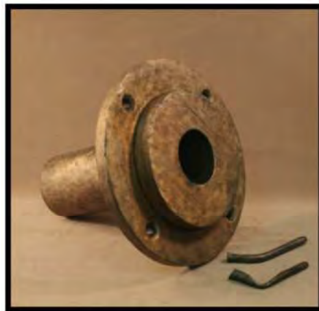
FIGURE 207. WESTFIELD DECK SOCKET FOR PIVOT CARRIAGE (ARTIFACT 122-046)
