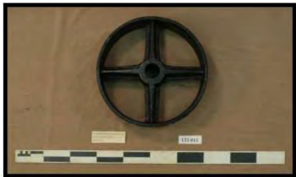
FIGURE 199. CAST IRON WHEEL FROM DONKEY ENGINE (ARTIFACT 132-011; SCALE CM/DM)
