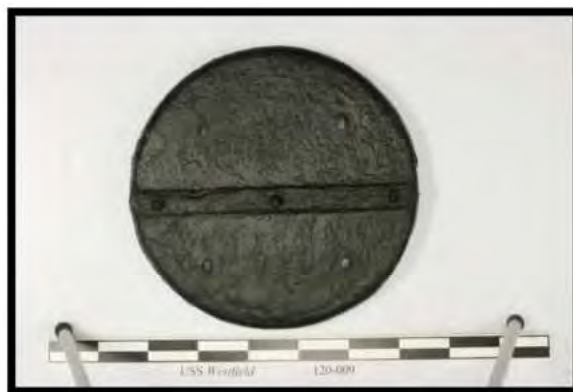
FIGURE 197. DOOR FROM HATCH ON REAR COMBUSTION CHAMBER (ARTIFACT 120-009; SCALE DM)
