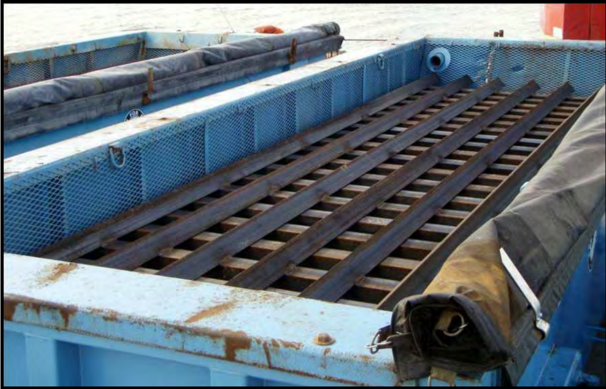
FIGURE 59. FILTER BOX WITH INSET 6-INCH MEC SCREEN INSERTED (PHOTOGRAPH BY SARA LAURENCE)
