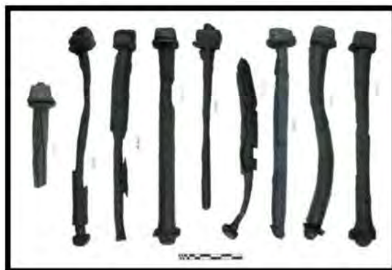
FIGURE 128. MASSIVE STAYBOLTS FROM UPPER STEAM DRUM (SCALE INCHES)
