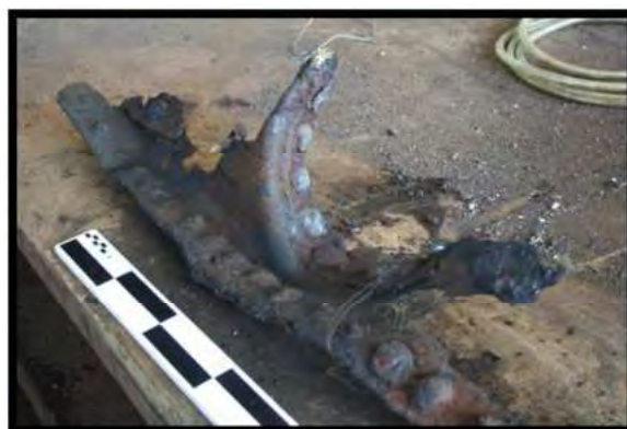
FIGURE 186. PLATING DESIGNED TO HOLD SMALLER ROUND FLUE (ARTIFACT 133-014; SCALE CM/DM)
