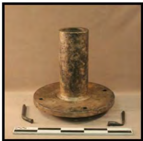
FIGURE 206. WESTFIELD DECK SOCKET FOR PIVOT CARRIAGE (ARTIFACT 122-046; SCALE CM/DM)
