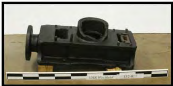
FIGURE 105. VALVE ASSEMBLY FROM AIR PUMP/HOT WELL RESERVOIR (ARTIFACT 132-017; SCALE DM)
