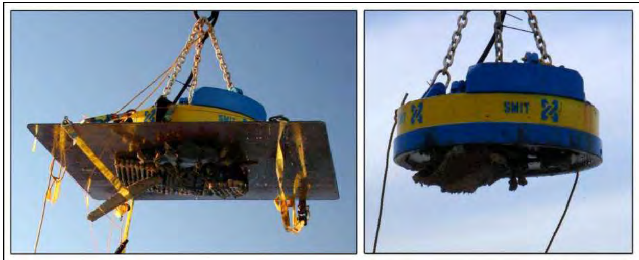
FIGURE 56. DETAIL OF ELECTROMAGNET (WITH AND WITHOUT ATTACHED PLATE)
