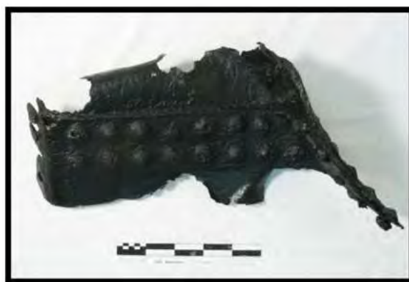
FIGURE 180. LOWER BOILER BARREL CONNECTION PLATES (ARTIFACT 133-011; SCALE CM/DM)
