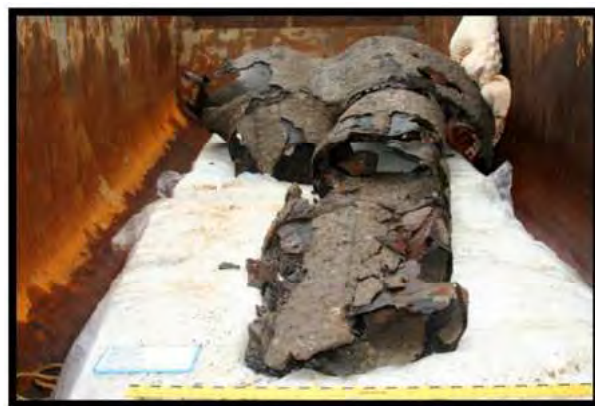
FIGURE 185. WESTFIELD 'S BOILER FLUES (ARTIFACT 122-001; SCALE INCHES)
