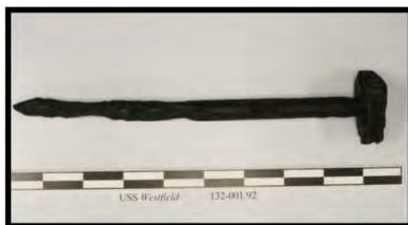
FIGURE 110. TYPE 2 MASSIVE BOLT FASTENER FOR CYLINDER BASE/BED FRAME TIMBERS (ARTIFACT 132-001.92; SCALE DM)
