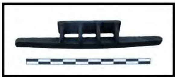
FIGURE 152. FORWARD BEARING BAR WITH "DEAD PLATE" (SCALE DM)
