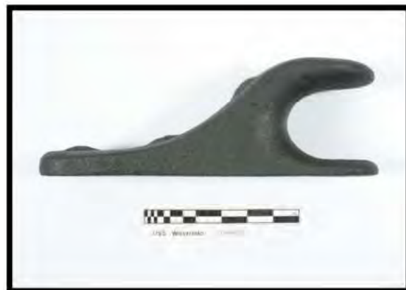
FIGURE 80. CAST IRON ROLLING CHOCK (ARTIFACT 125-068; SCALE INCHES)
