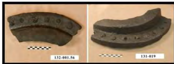
FIGURE 145. FRAGMENTS OF MAN HOLE FRAME FROM TOP OF BOILER BARREL (ARTIFACTS 131-019 AND 132-001.56)
