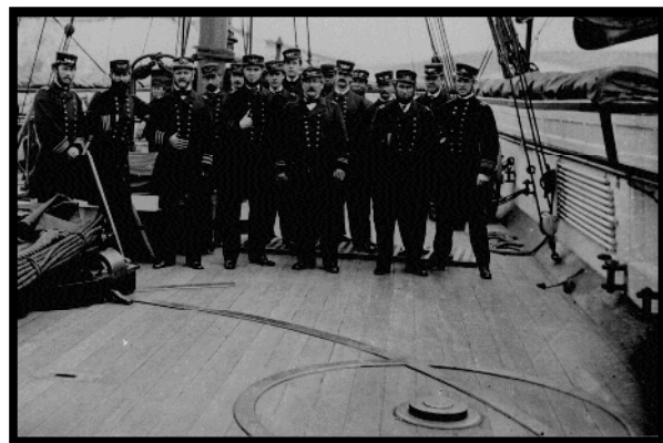
FIGURE 208. SOCKET FOR PIVOT CARRIAGE IN DECK OF UNIDENTIFIED GUNBOAT.
