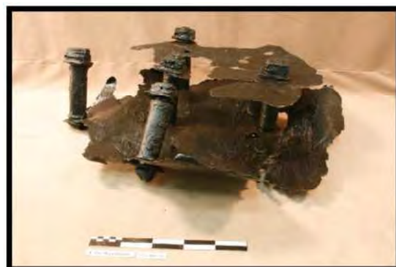
FIGURE 192. UPPER FRAGMENT OF COMBUSTION CHAMBER (ARTIFACT 132-001.76; SCALE CM)
