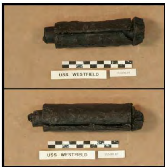
FIGURE 147. EXAMPLES OF FIRE BOX STAYBOLTS (ARTIFACTS 132-001.64 AND 132-001.67)
