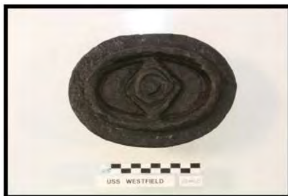
FIGURE 139. SMALLER SIZED HAND HOLE CLEANING COVER (ARTIFACT 132-001.55)
