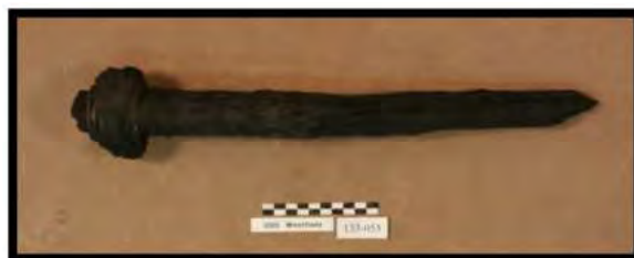
FIGURE 115. ROD ARTIFACT WITH THREADED BRASS BUSHING (ARTIFACT 133-053)
