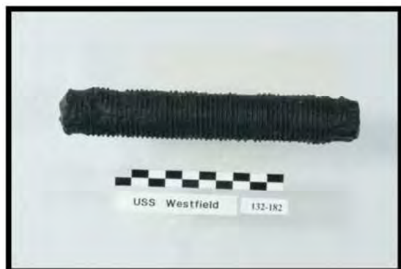
FIGURE 191. THREADED STAYBOLT WITH HAMMERED ENDS (ARTIFACT 132-182)
