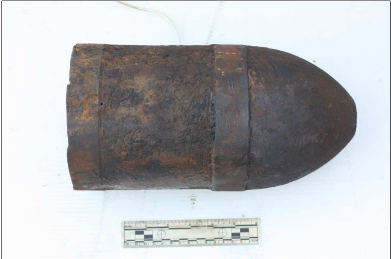
Figure 6-386. Brooke 6.4-inch ratchet disc sabot shell, Artifact 2364.13, during electrolysis. Note the ratcheted end, left, and the bourrelet band center.
