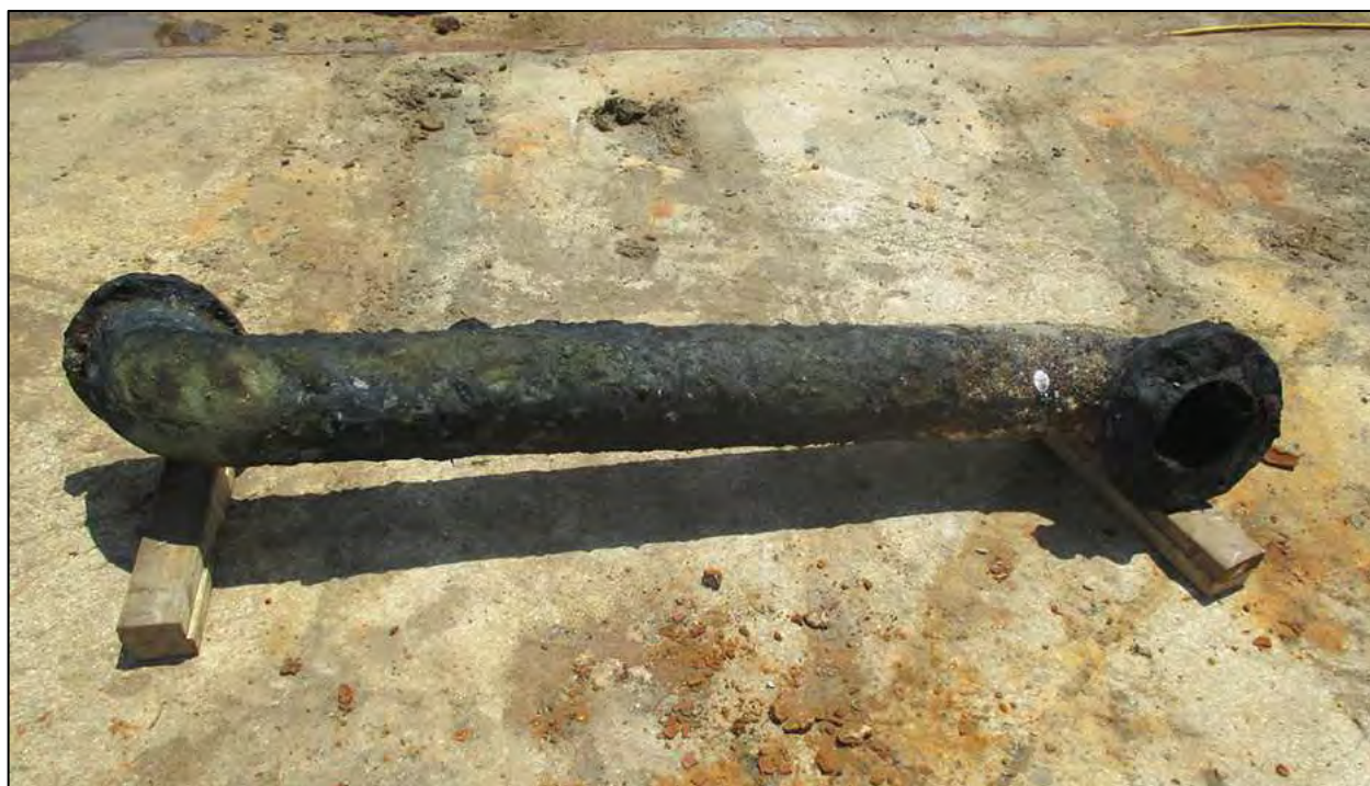
Figure 6-56. Iron steam pipe recovered during Large Artifact Recovery. The ends of the 5-foot pipe are bent 90 degrees in opposite directions and fitted with 12-inch diameter flanges. The flanges are drilled for five bolts and gaskets; several bolts survive.
