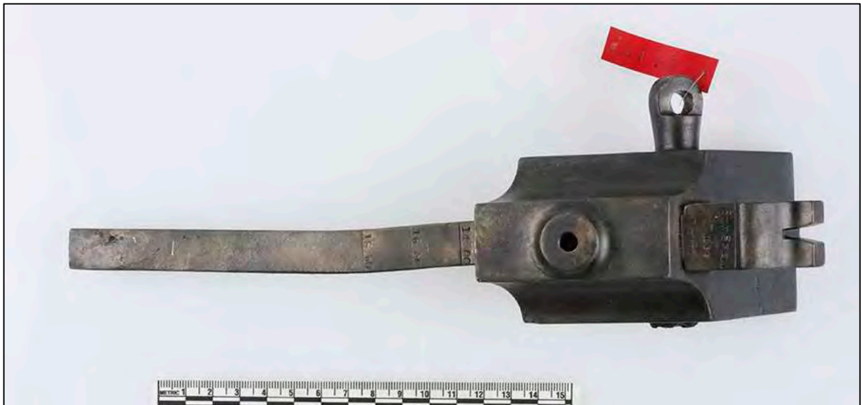
Figure 6-318. Artifact 1856.10 - W. of "box": 2.3 in. (5.8 cm), Diameter of screw hole: 0.3 in. (0.8 cm), W. of tangent scale: 0.6 in. (1.5 cm), L. of tangent scale: 10.5 in. (26.7 cm). Typical tangent sight. Tangent scale slightly bent. Largest graduation is 1860. Stamps on head read: 8 IN. SHELL, 7 LBS. LEVEL. Stamps on "box" read: NO: 112 8 IN. 56 CWT.
