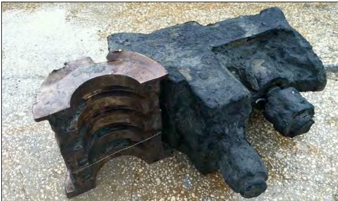
Figure 6-485. Recovered from G-125, Artifact 1909.05, a bearing pillow block recovered from Unit 6-E and half of a four-collared bronze thrust bearing recovered from the same grab that would have attached to the propeller shaft.
