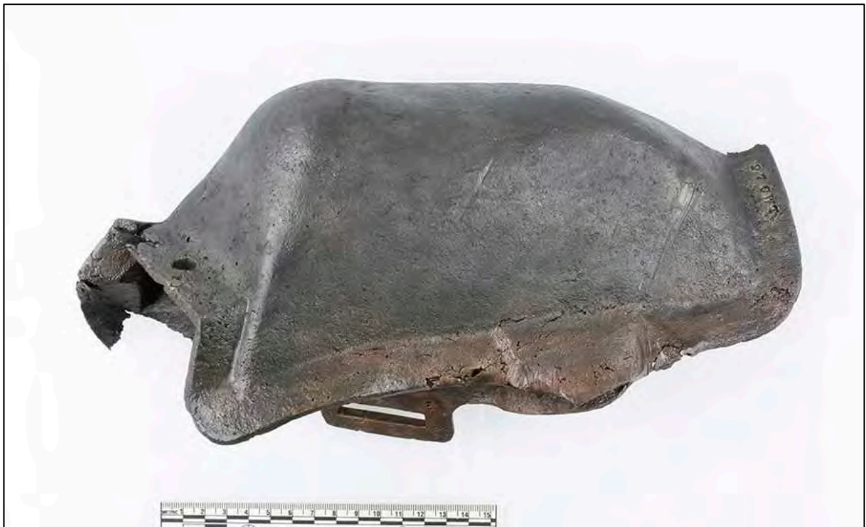
Figure 6-322. Artifact 1850.17 – Tangent cover - Length 12.3 in. (31.2), Width of narrow opening on side: 0.3 in. (0.8 cm). Extremely distorted. Stamp on outer edge reads: 27 CWT.
