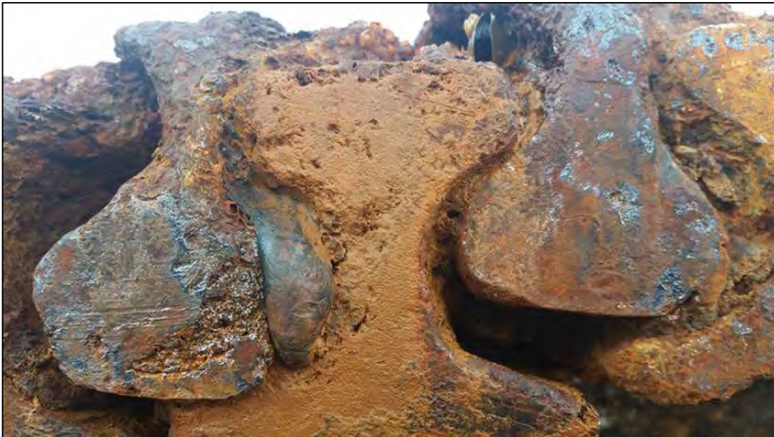
Figure 6-520. Close up of rails showing four different rail shapes. Also note the black pitch which has oozed out due to heat and possible filler to the right, both may represent “...a composition of iron filings and some kind of cement...laid upon the irons so as to cover the inequalities and to make it solid and keep it from shaking” (Swanson and Holcombe 2003:74).
