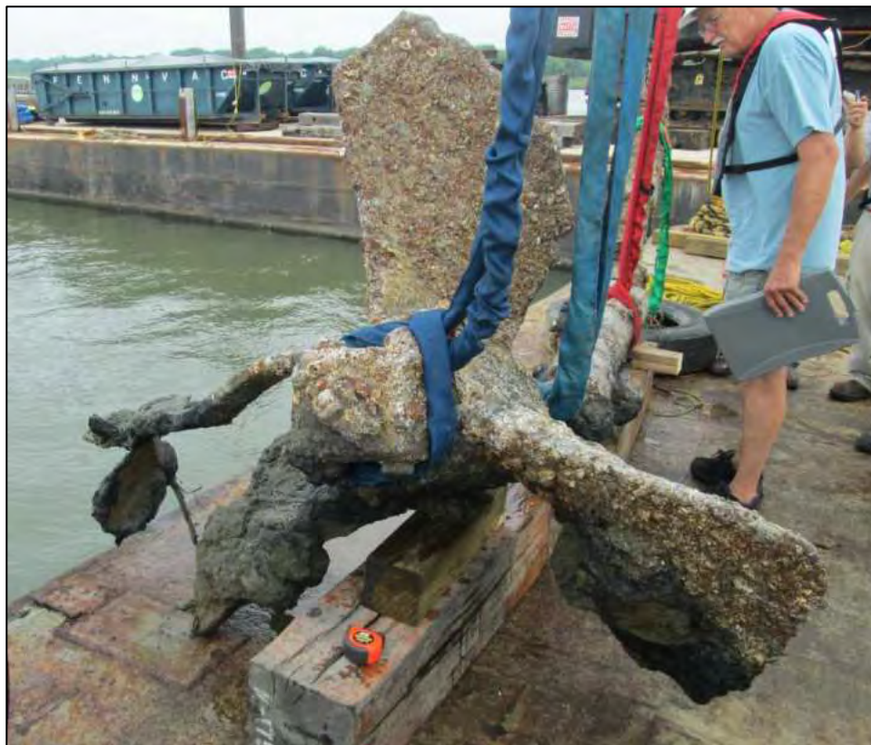
Figure 6-479. End view of propeller showing the hub shaft bushing (center) and remaining strut mount (left).
