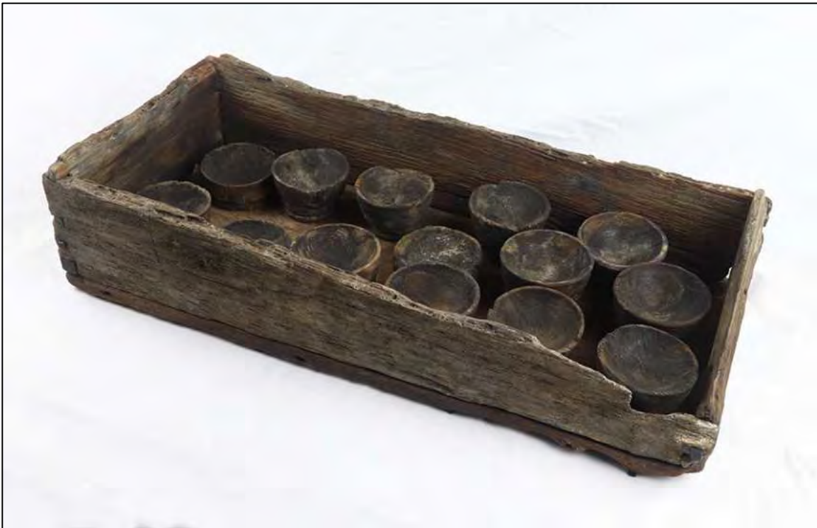
Figure 6-411. The 14 6-pounder sabots after conservation, showing both predominant tall conical type and the three examples of the short cylindrical form, Artifact 3264.1.
