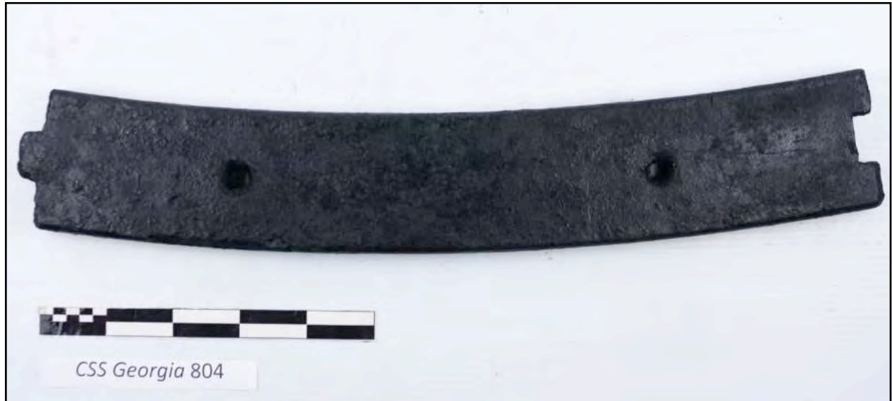
Figures 6-359. Section of pivot-carriage track recovered from Unit 10-E (Artifact 804). Note the notches at either end for fitting pieces together, as well as holes for fastening track pieces to the deck.
