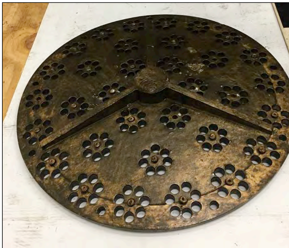
Figure 6-506. Artifact 1861.13, a Worthington direct-acting steam pump plate, bronze valve plate after conservation, base view. The iron covering would have attached to this side.
