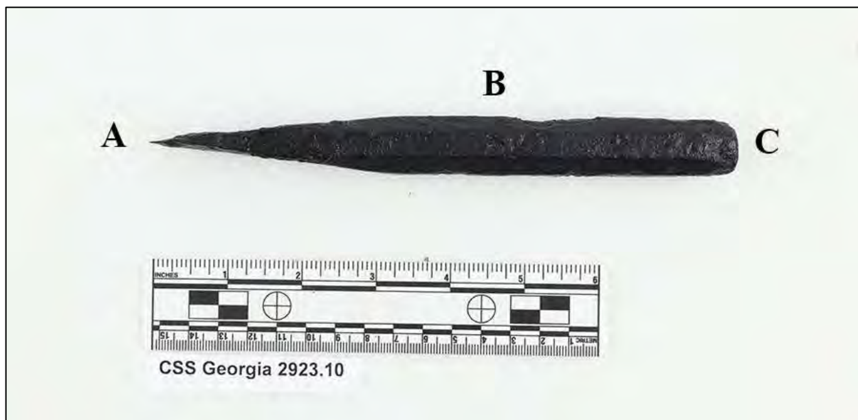
Figure 6-228. Artifact 2923.10 cold chisel parts as follows: (a) bit, (b) stock, and (c) head (courtesy of CRL Texas A&M University). “Bit” follows Light (2007:105), whereas “Stock” and “Head” follow Scientific American (1884:32).
