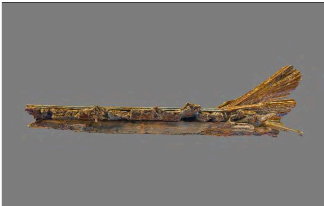
Figure 6-514. Orthomosaic of East Casemate end view, casemate base at left, top at right. Rail is on top of and fastened to 8-inch thick horizontal oak that was attached to 12-inch thick vertical pine timbers (at bottom). The large pine timbers formed the interior wall of the ironclad.
