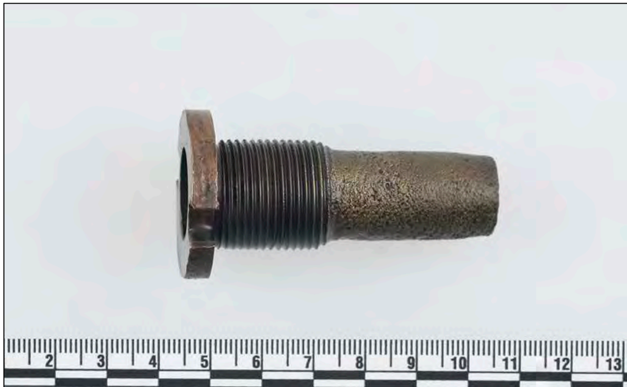
Figure 6-397. Alger pattern naval water-cap time delay fuze from the spherical IX-Inch Dahlgren shell above, Artifact 1983.30.
