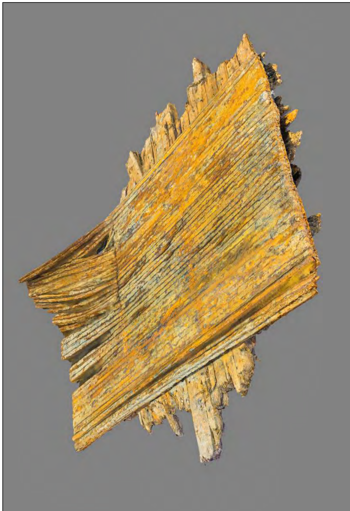
Figure 6-94. 3D isometric of the main section of the East Casemate. Note the bent rails and where they break at the line of fasteners.
