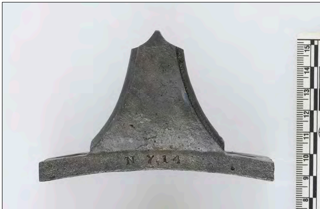
Figure 6-325. Artifact 1856.14 (1 of 2) - Height: 2.4 in. (6.1 cm), W. of base: 1.4 in. (3.6 cm), L. of base: 3.9 in. (9.9 cm). Typical dispart sight. Tallest in the collection. Stamp on base reads: 714.
