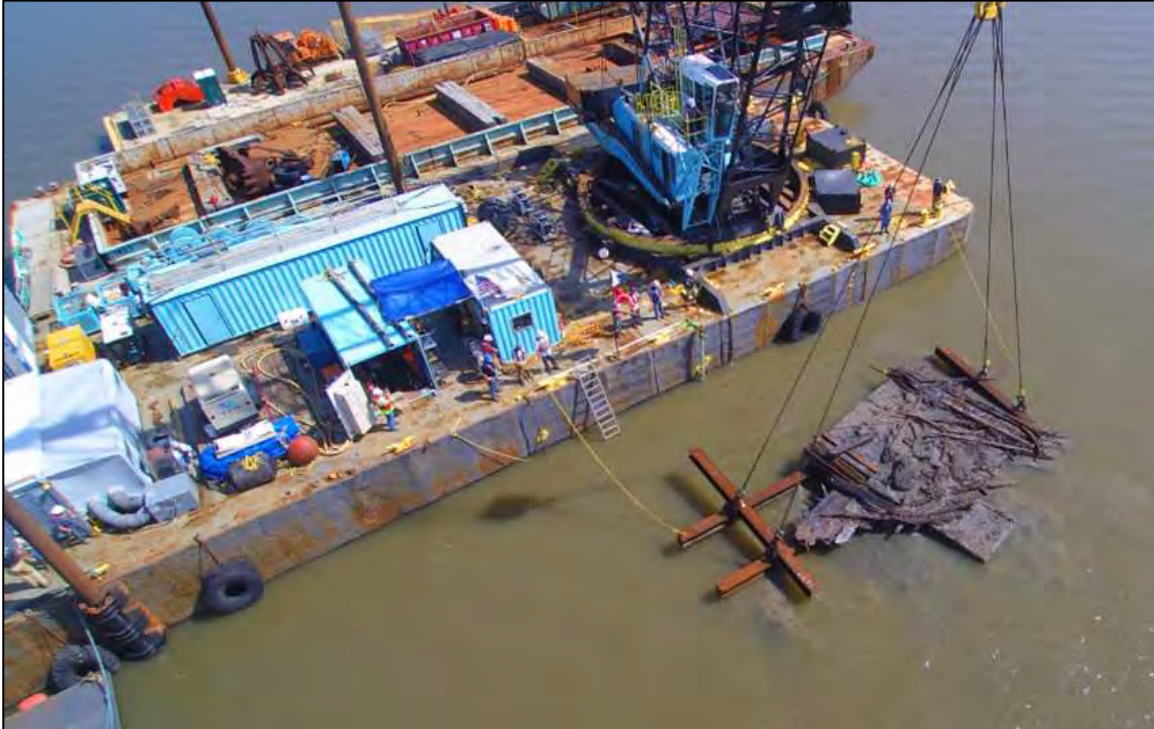
Figure 6-100. Drone shot of West Casemate lift just breaking the surface. At this point it was found to weigh 40 tons without the lift frame. It will be lifted and swung around to the middle Witte barge (middle barge) where it will be placed on wooden bunks next to the East Casemate. Note the dive station CONEX box to the left of the crane, and grey command tent to the far left.
