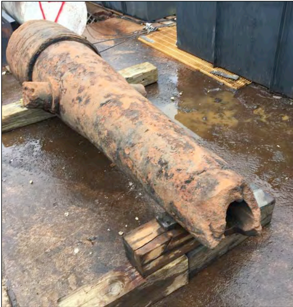
Figure 6-296. 6.4-inch Brooke rifle, Cannon No. 4, Artifact 1613 taken out of electrolysis for analysis. As a result of one of two muzzle explosions aboard the CSS Georgia thought to be the result of defective shells, the remaining length is just under 10 feet.
