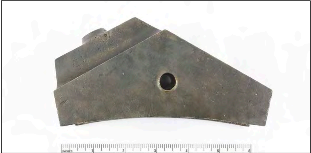
Figure 6-321. Artifact 2997.4 – Side View. Length 5.8 in. (14.8 cm), Width 2.5 in. (6.4 cm), Diameter of screw hole: 0.3 in. (0.8 cm), Width of scale opening: 0.5 in. (1.3 cm). Shape resembles that of the previous sight “boxes” from previous tangent sights except for CSSG 978. Barely any damage, no marks, no stamps.
