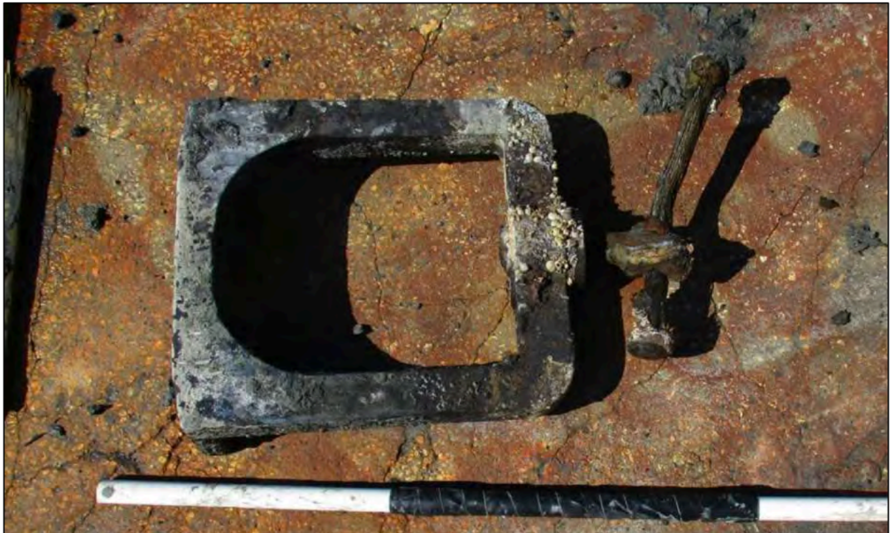
Figure 6-347. Carriage compressor immediately after mechanized recovery from G-15. Note the still intact compressor screw and tightening rod.
