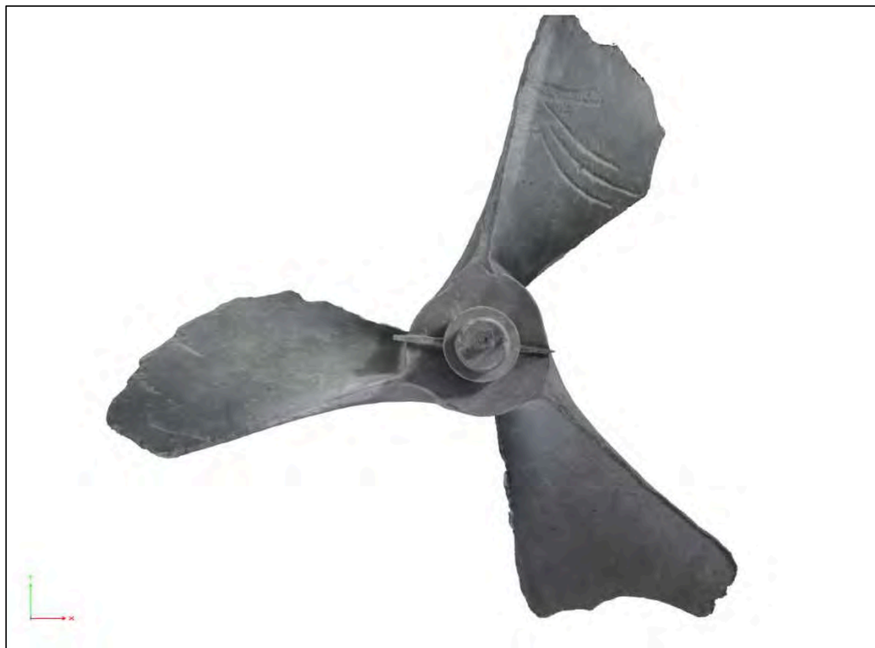
Figure 6-480. 3-D end-on image of Artifact 1614, a triple-bladed propeller recovered from Unit 2-F. Note the broken blades. Shaft bushing and strut mounts removed during conservation; shaft bushing in center of the shaft.
