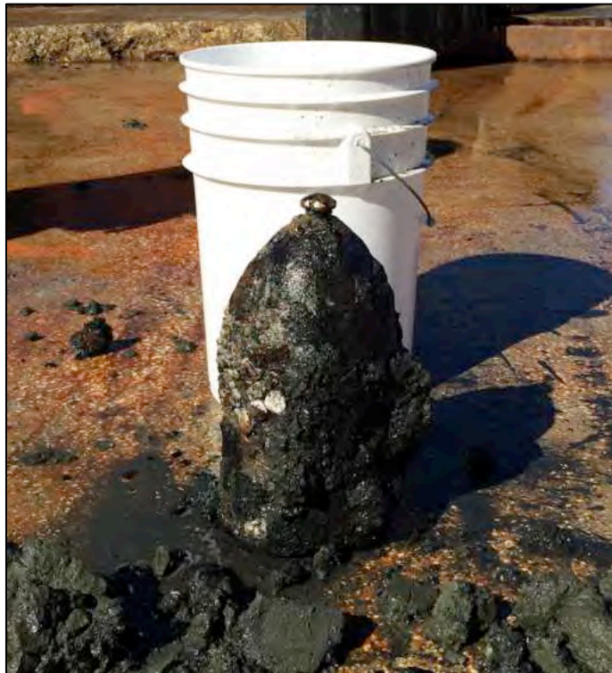
Figure 6-380. Brooke shell recovered with Grab G-482, photographed prior to placement in bucket. The shell and small amount of sediment were all that were recovered with Grab G-482. Note the shell's shiny brass Archer fuze.
