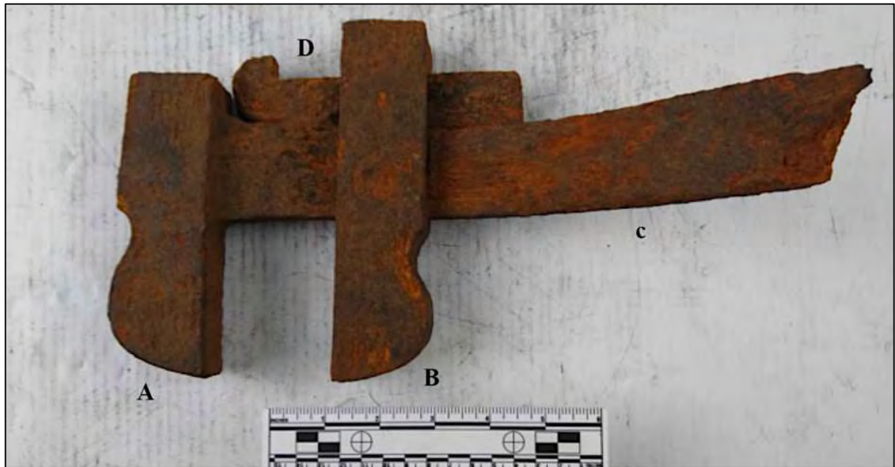
Figure 6-245. Artifact 1899.20, an adjustable wrench, parts as follow: (a) upper jaw/fixed jaw, (b) lower jaw/moving jaw, (c) bar, and (d) gib wedge. Because some parts of this adjustable wrench are functionally comparable to screw wrench Artifact 1879.19, labels (a), (b), and (c) follow Artifact 1879.19, while (d) is taken from Richardson (1890:42; courtesy of CRL Texas A&M University).
