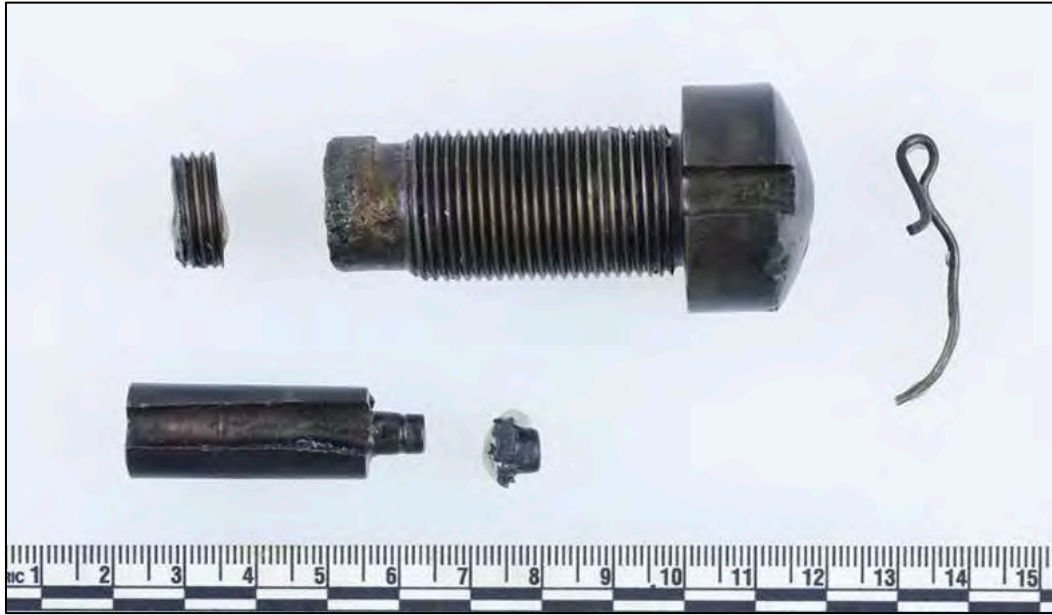
Figure 6-391. Archer safety pin percussion fuze from CSS Georgia after conservation showing all components. Artifact 4091 from Brooke Shell Artifact 4091. Internal slide with percussion cap at bottom.
