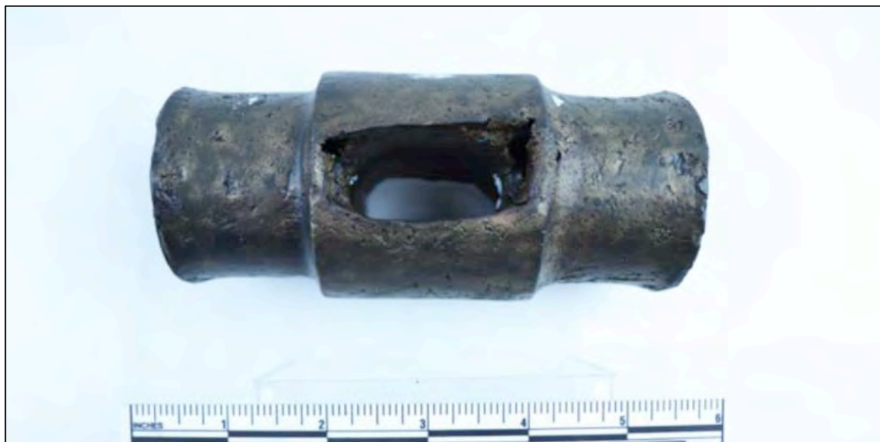
Figure 6-232. Artifact 1899.2 is an anti-sparking brass hammer (courtesy of CRL Texas A&M University).
