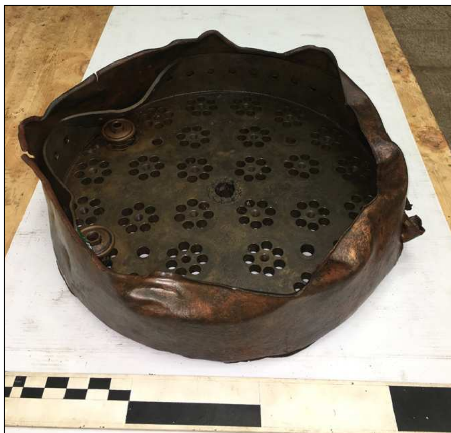
Figure 6-505. Artifact 1861.13 after conservation. Shown are the Worthington direct-acting steam pump copper housing with bronze valve plate. Two valves have been reinserted.
