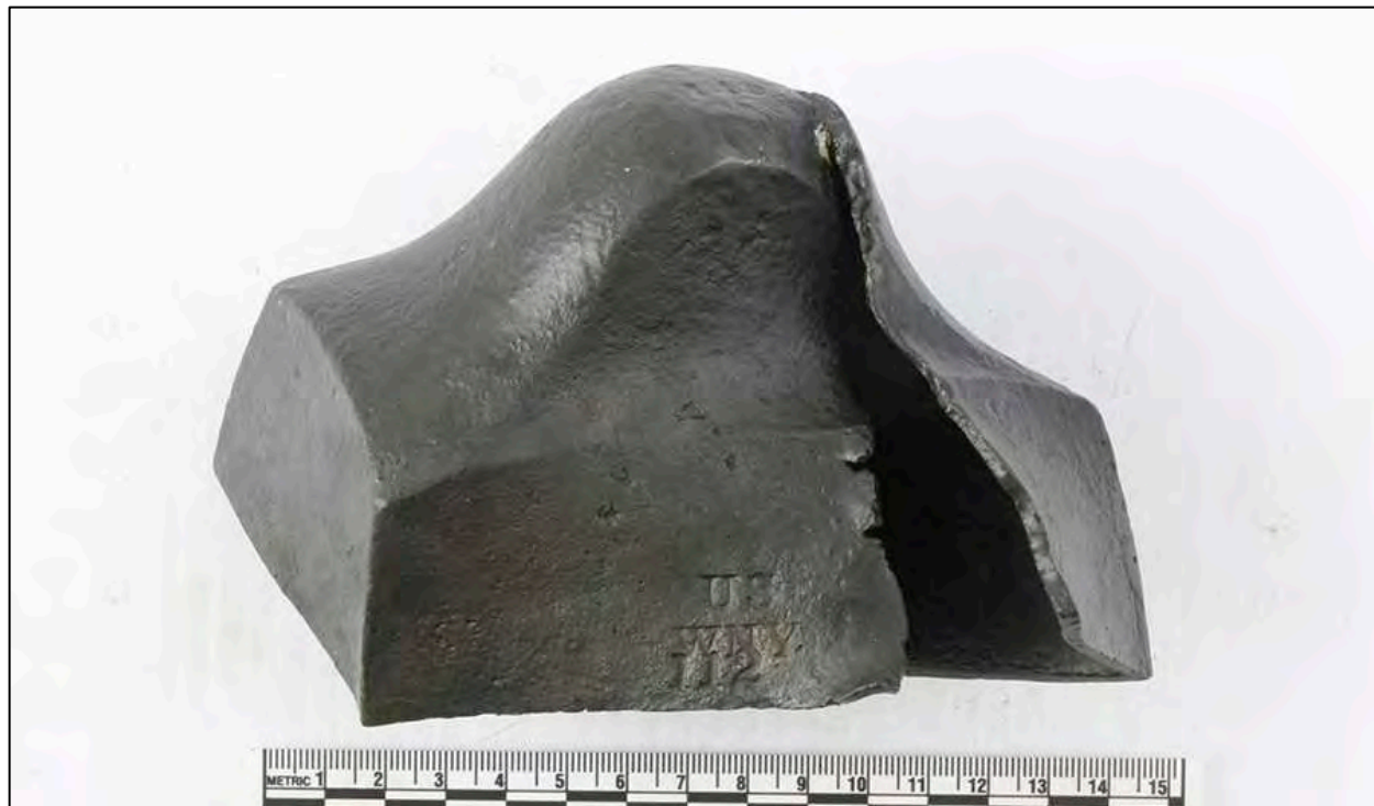
Figure 6-328. Artifact 1881.28 - Max. height: 3.9 in. (9.9 cm), Max. length: 6.3 in. (16.0 cm). Dispart sight cover. Shape is distorted. Stamp on base reads: US WNY 112. Stamp at the top reads: 112.
