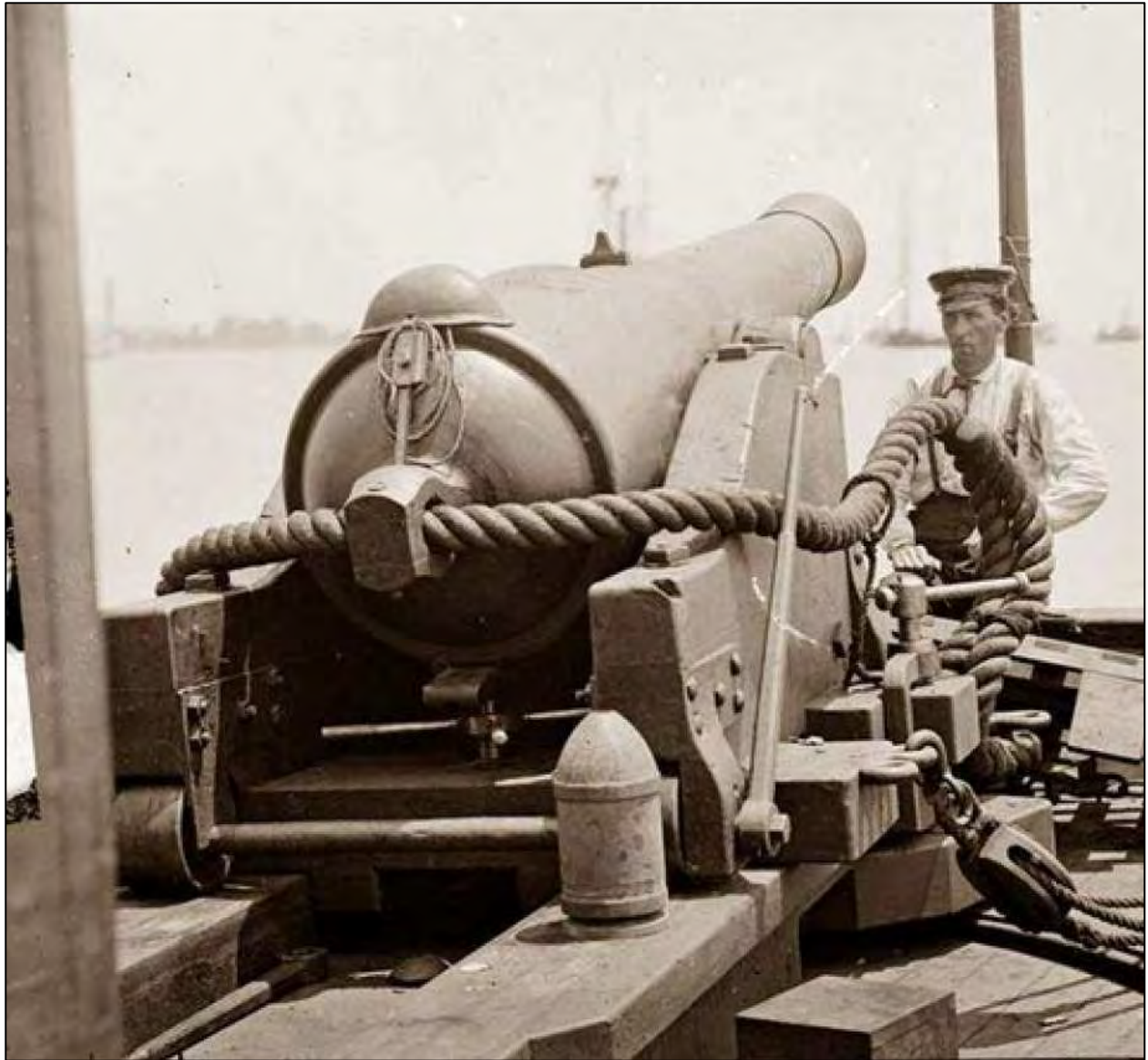
Figure 6-338. Brooke Rifle and pivot carriage on the CSS Teaser (Miller and Lanier 1911:77).
