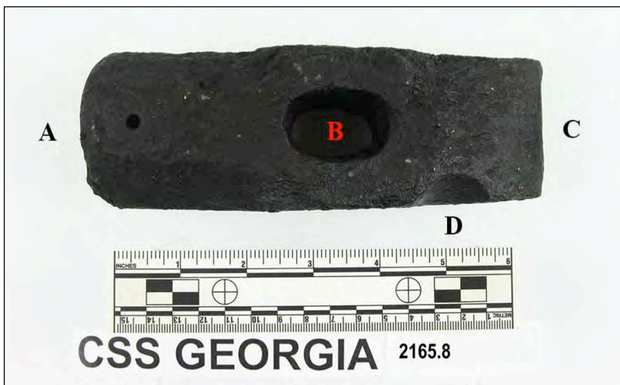
Figure 6-233. Cross-pein sledgehammer hammerhead parts as follows: (a) face, (b) eye, (c) pein, and (d) chamfer (courtesy of CRL Texas A&M University). Labels follow terminology in Blackburn (2000:67).
