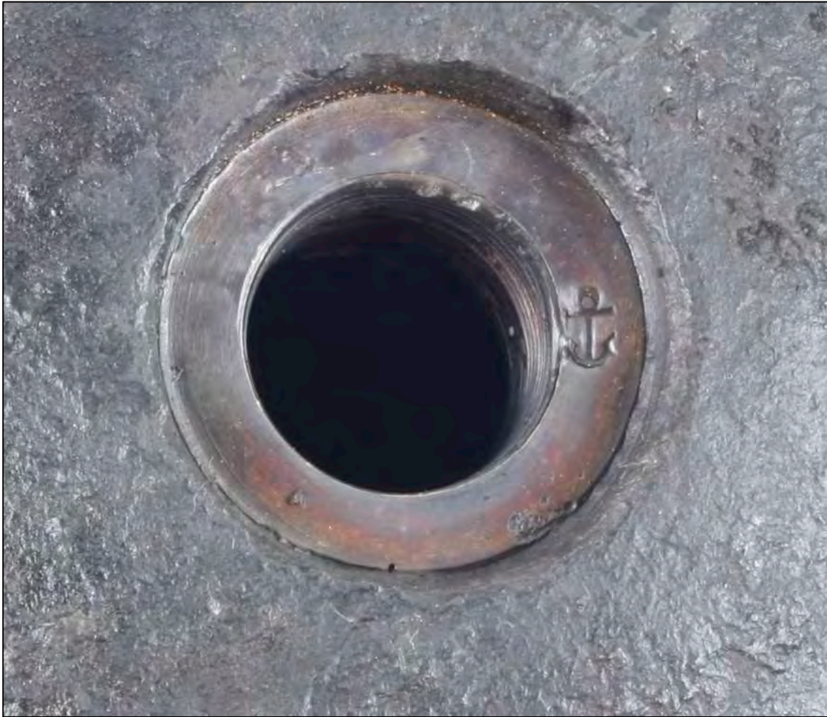
Figure 6-3954. Anchor stamp in the fuze well bushing of a spherical IX-Inch Dahlgren shell.
