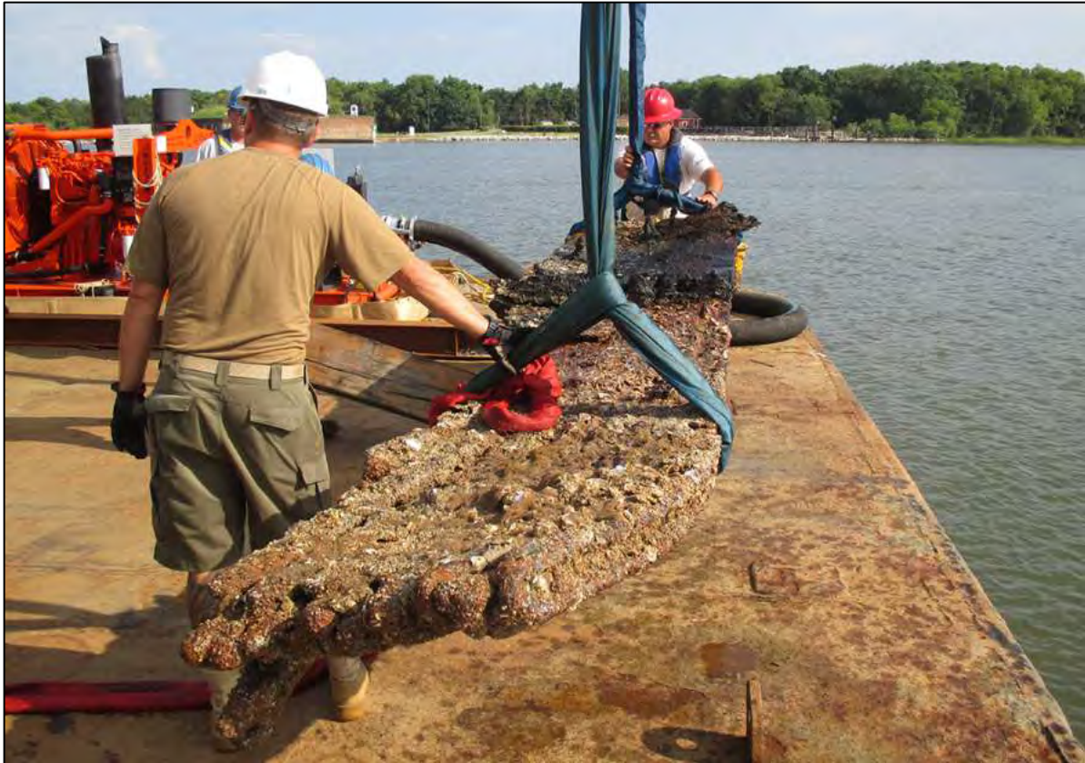
Figure 6-72. The third section raised (No. 3). This piece calved off a smaller rectangular section when lifted. Note that the rails are bent on the upper end. Not an as-built feature, this bending is also noted on portions of the West Casemate rails, possibly a result of salvage or later pre-data recovery impact.
