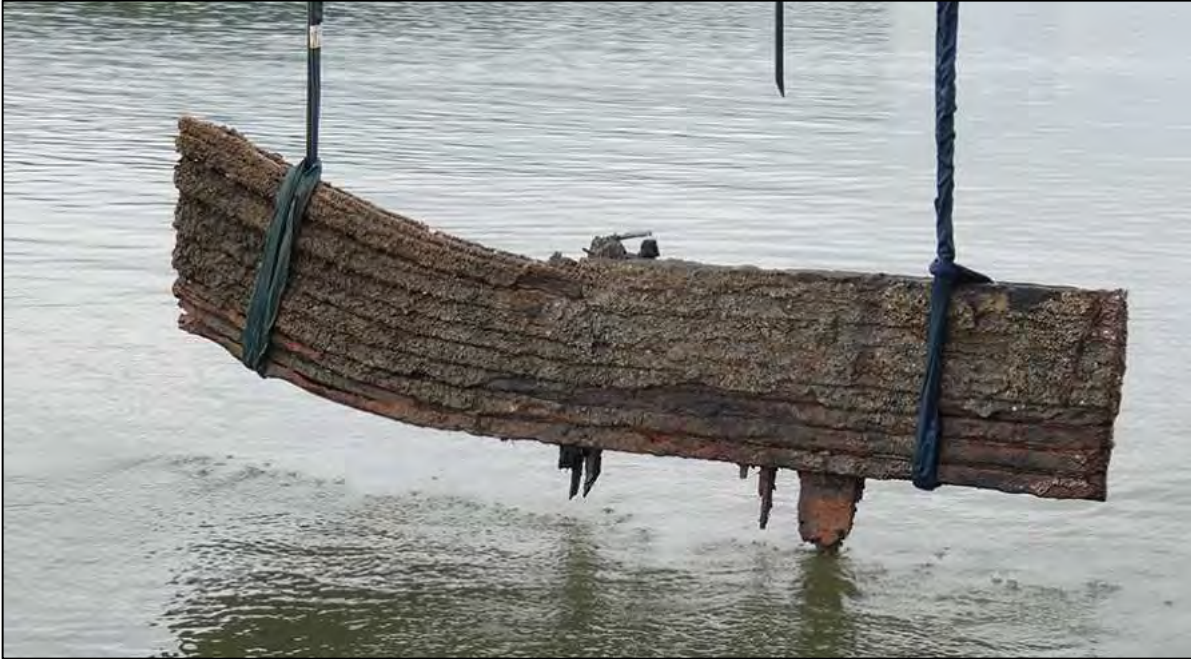
Figure 6-83. Larger (No.1) section recovered from the West Casemate. Note the bent rails at left, a feature clearly seen in Figure 6-77. Not an as-built feature, this bending was also noted on portions of the East Casemate rails, possibly a result of salvage or later pre-data recovery impact.
