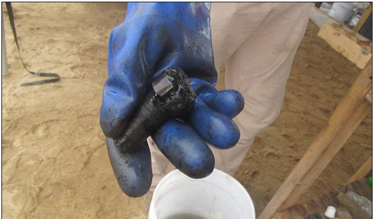
Figure 6-44. Archer fuze that has just been removed from a 6.4-inch Brooke shell (courtesy of the U.S. Army Corps of Engineers–Savannah District).
