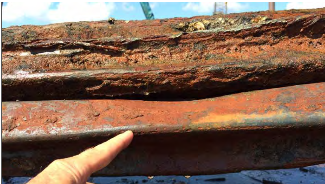
Figure 6. Note bend in railroad iron from blade on edge of southern segment recovered from East Casemate.
