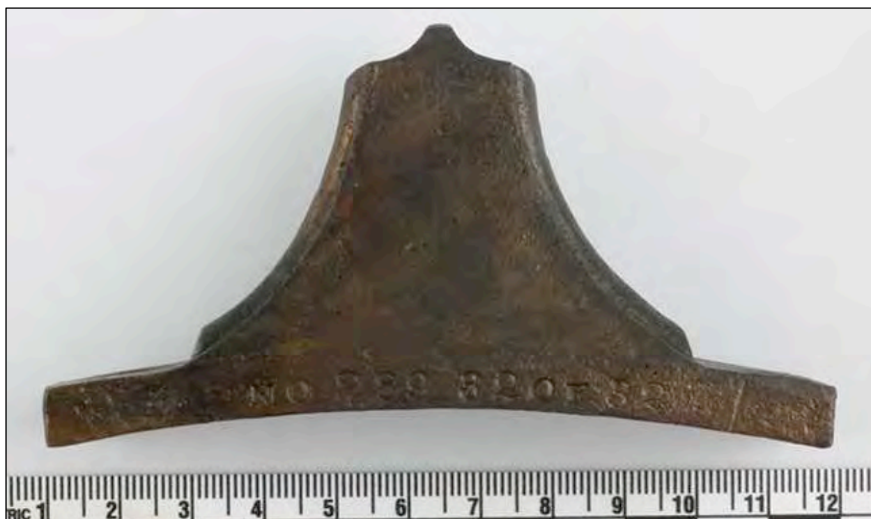
Figure 6-323. Artifact 2994.8 - Height: 2.0 in. (5.1 cm), W. of base: 1.3 in. (3.3 cm), L. of base: 4.0 in. (11 cm). Typical dispart sight. Stamp on the base reads: NO. 289 32 of 32 meaning 32 sights were made in that "batch."
