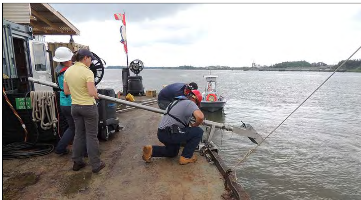
Figure 6-28. CODA sonar head being readied next to the Dive Station. By turning the pole, the sonar head was easily directed to anywhere coverage was required.
