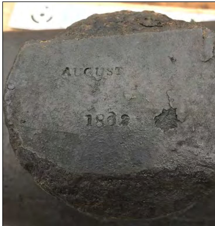
Figure 6-281. Left trunnion of recovered 6-pounder cannon marked August 1862. Observe the “6” in 1862 is reversed left to right. The only way to accomplish this error is to use a foundry pattern stamp, which is reversed for use on molds.
