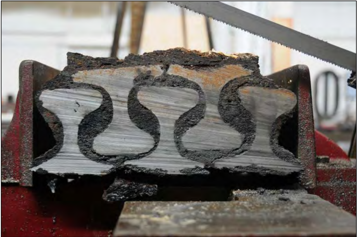
Figure 3-20. Initial profile cut of the small section of rail required for subsequent testing. This cut took six hours. Note that the rails look to be in excellent condition, with only minimal metal loss due to corrosion.
