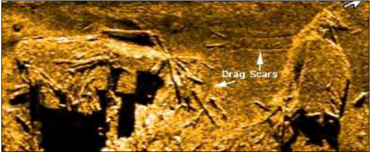
Figure 5-15. 2003 acoustic image of the West (left) and East (right) Casemate sections. Note the two linear drag scars at the top left of the East Casemate projecting toward the West Casemate, and a second fainter set running toward the channel to the right of the West Casemate. Also note 6-pownder cannon to the right of the East Casemate's midsection.
