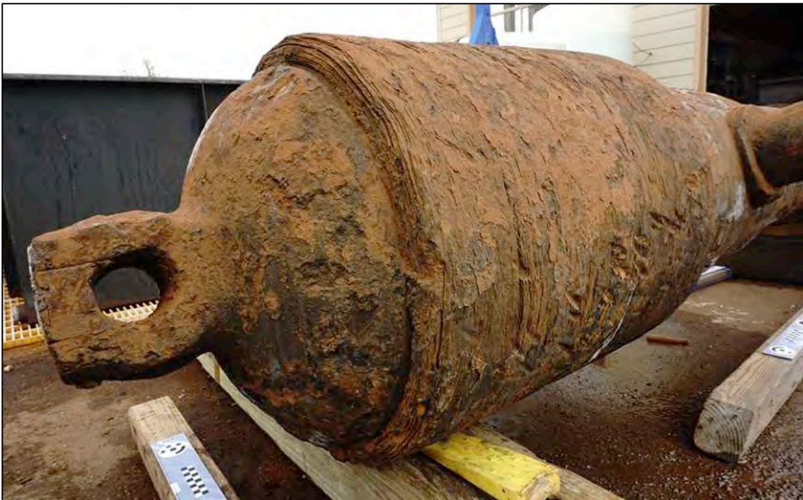
Figure 6-298. Breech of 6.4-inch Brooke rifle, Cannon No. 4, Artifact 1613 showing layered wrought iron breech banding in relationship to the cast iron of the cannon tube. Note the similarity to the insert completing the circular opening for rope of Cannon No. 2 (Artifact 1612) in Figure 6-288.
