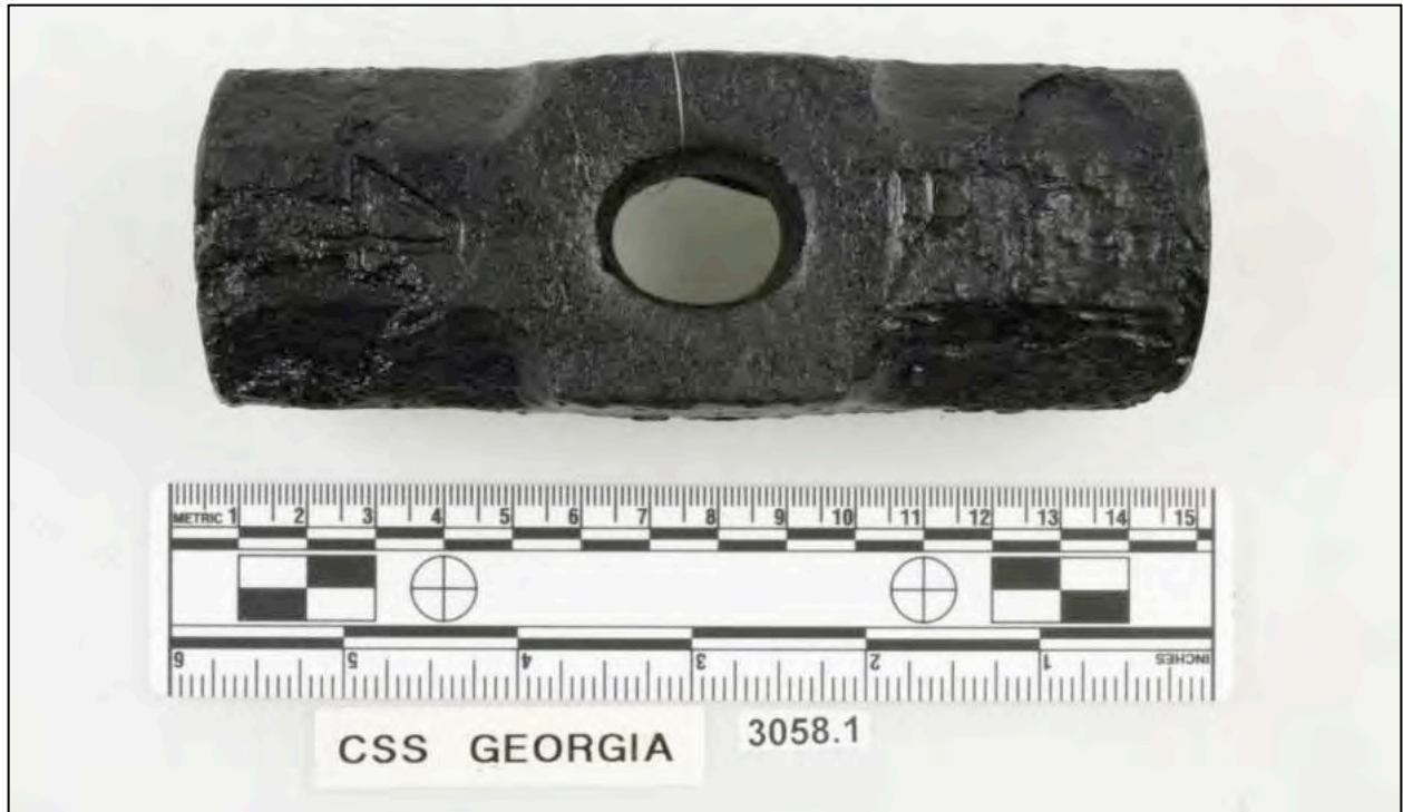
Figure 6-235. Artifact 3058.1 is a “double-faced” or “engineer’s” hammer. Note that the scale bar is positioned with metric at top in this photo (courtesy of CRL Texas A&M University). Note the cast “4” at left.
