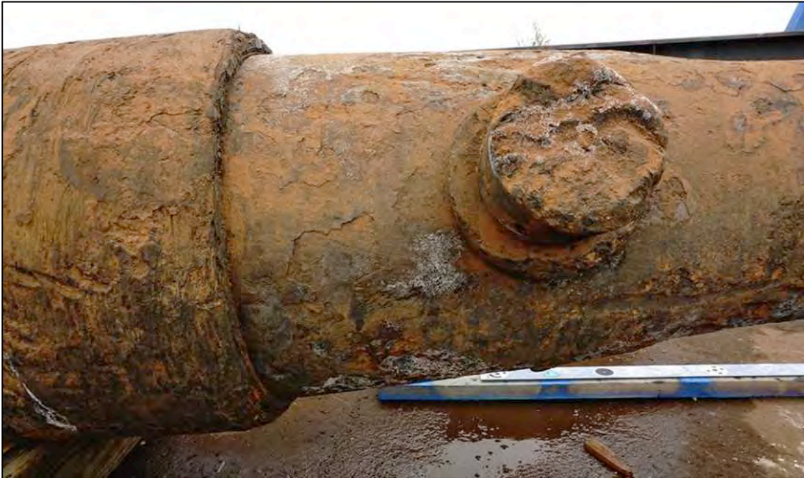
Figure 6-297. Right trunnion of 6.4-inch Brooke rifle, Cannon No. 4, Artifact 1613 showing extreme corrosion precluding observation of foundry markings.
