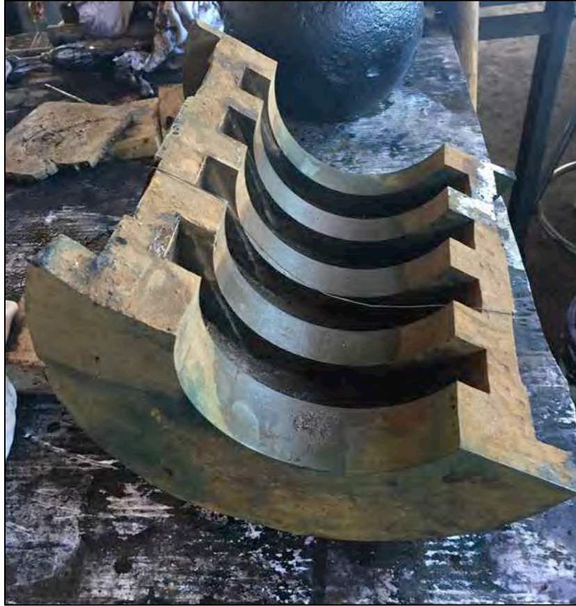
Figure 6-487. Internal view of half of four-collared bronze thrust bearing.
