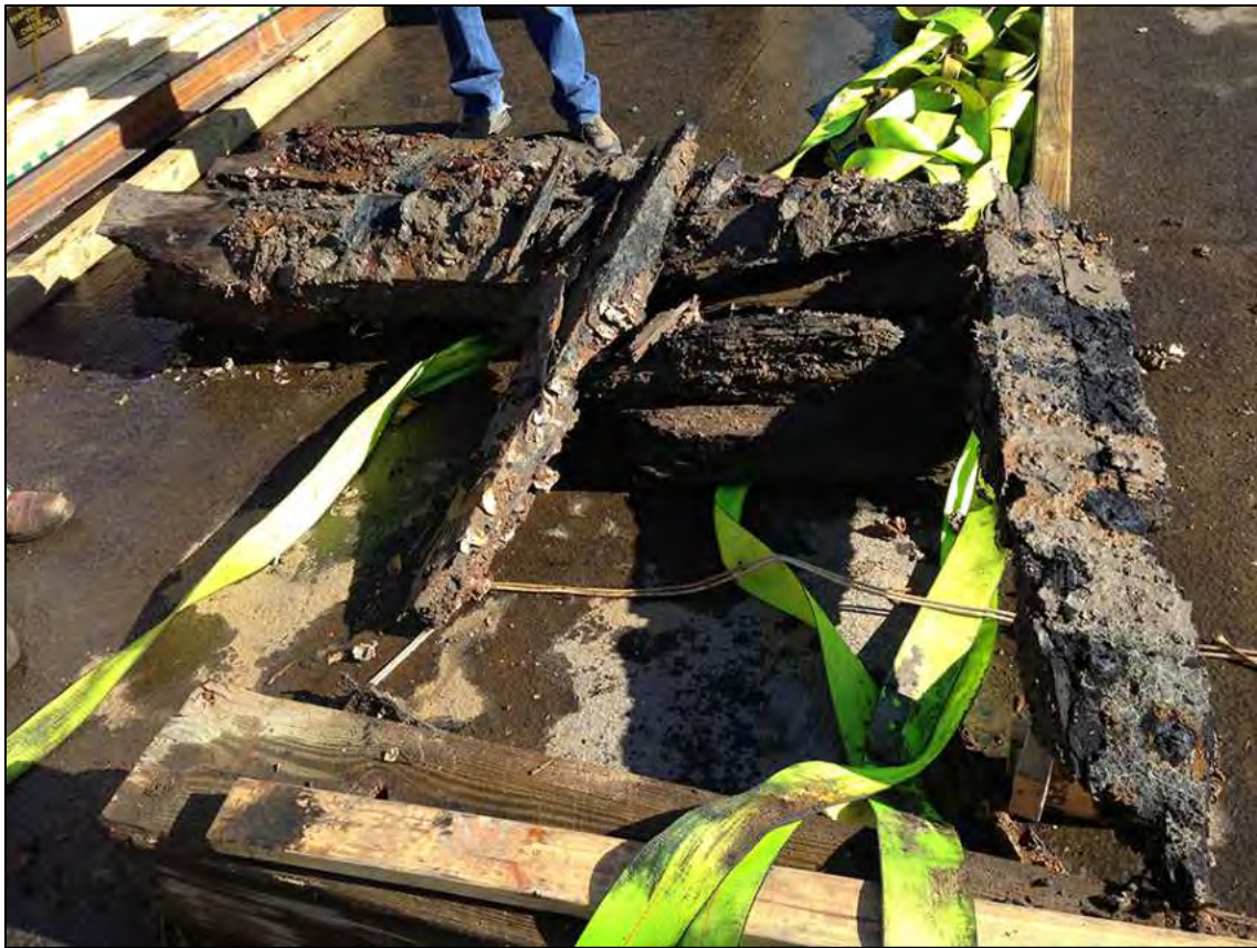
Figure 3-18. Wood backing that detached from the Recovery Section. The wood for the most part was in a highly deteriorated condition with little integrity that fell away from the iron rails when unsupported.
