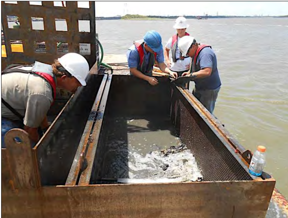
Figure 6-107. With the large 6-x-6-inch top grate raised, personnel had to enter the screen to wash sediment through two horizontal grates. The weight of the grates made them difficult to lift and clean, and the position of the screens was found to be inadequate, with numerous limitations on processing (i.e., removal of sediments, etc.).
