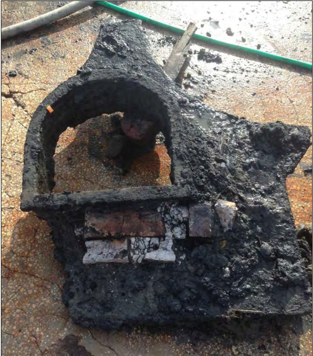
Figure 6-257. Firebrick still attached to the inside of the boiler face just below one of the doors. Notice the white and cracked nature of the brick, indicating extreme heat. Artifact 1844.02 is from Unit 6-E just south of the West Casemate.
