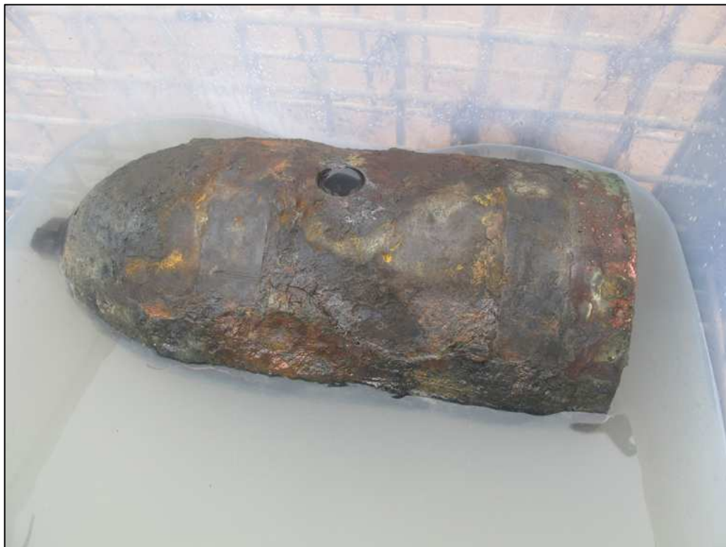
Figure 6-45. Inerted Brooke shell with hole drilled for removal of all contents. Note the fuze has not yet been removed (courtesy of the U.S. Army Corps of Engineers–Savannah District).
