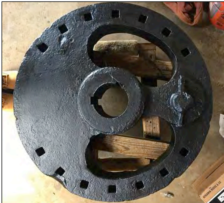
Figure 6-490. Conserved Artifact 1899.17, a counterbalance flywheel recovered from Unit 6-C. Three feet in diameter and 5 inches thick, this is the opposite side from Figure 6-490.
