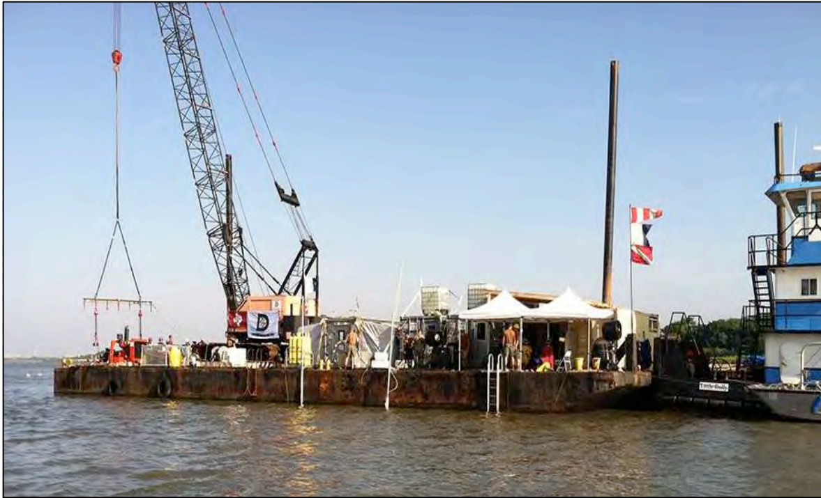
Figure 6-25. The smaller barge with 75-ton crane. The Command Center is immediately to the right of the crane. The Dive Station is far right, marked by a dive ladder and two white tents. CODA system and equipment rooms are in CONEX boxes between the Dive Station and Command Center. The CODA system pole is to the left of the dive ladder, with the USBL transponder pole to its left. The CONEX box at far right next to dive flags holds a recompression chamber.
