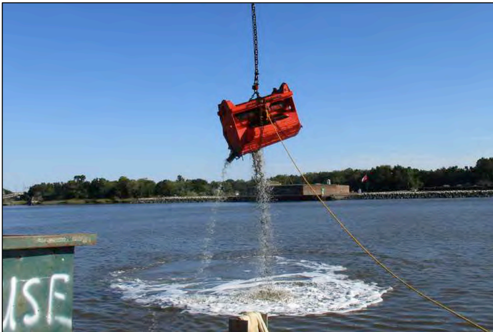
Figure 6-105. Clamshell grab being brought on board. Notice the timber disallowing closure of the mouth, with a resultant loss of sediment.
