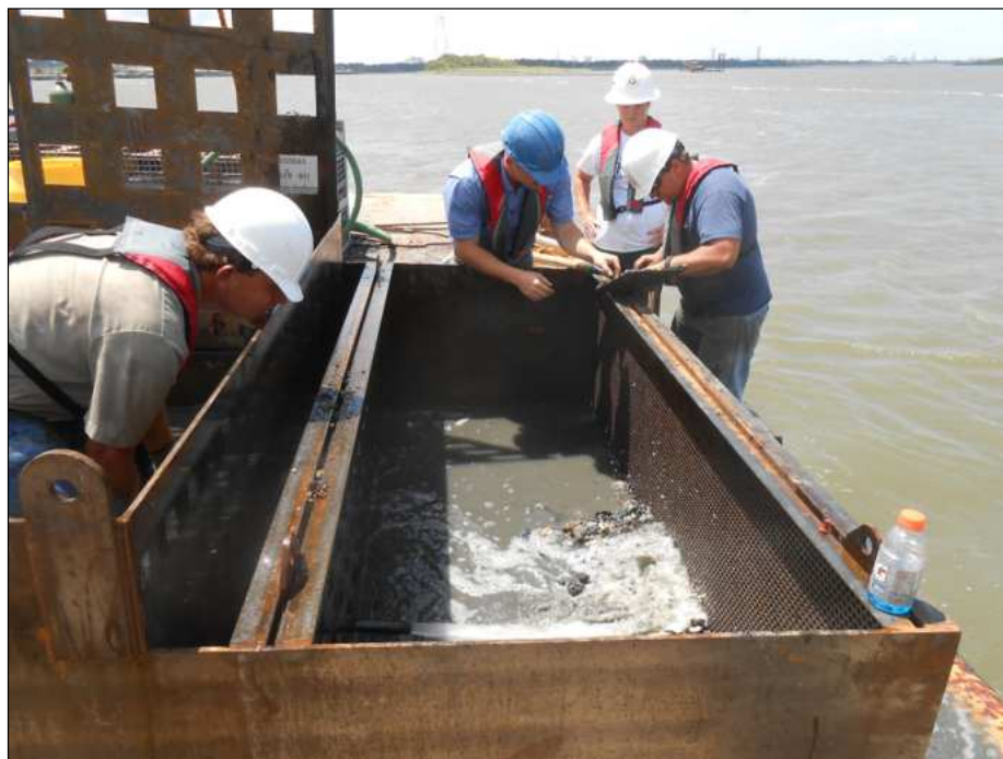
Figure 13. With large 6 x 6 inch screen raised, washing sediment through 2 horizontal screens. Weight and positioning of screens was found to be inadequate with numerous limitations on processing.
