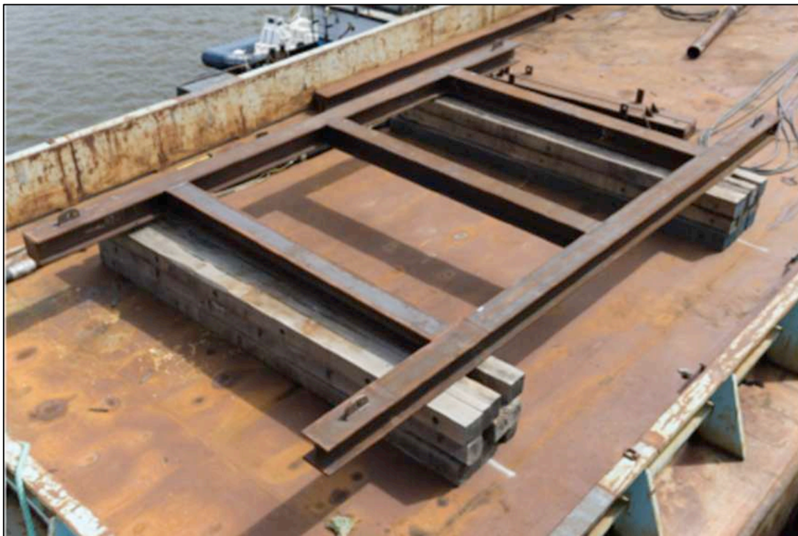
Figure 6-87. Iron I-beam frame for lifting casemate sections.
