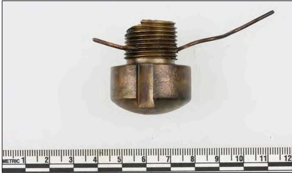
Figure 6-392. Side view of a conserved but broken Archer fuze showing the position of the safety pin or wire, Artifact NP5.
