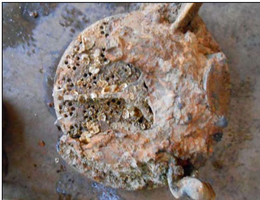
Figure 6-504. Opposite side of the Worthington direct-acting steam pump, Artifact 1861.13. The bronze plate with its valve holes can be seen underneath the concreted iron in Figure 6-505.
