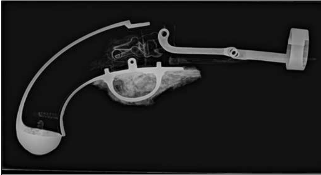
Figure 6-425. Pre-conservation X-ray image of the pistol.
