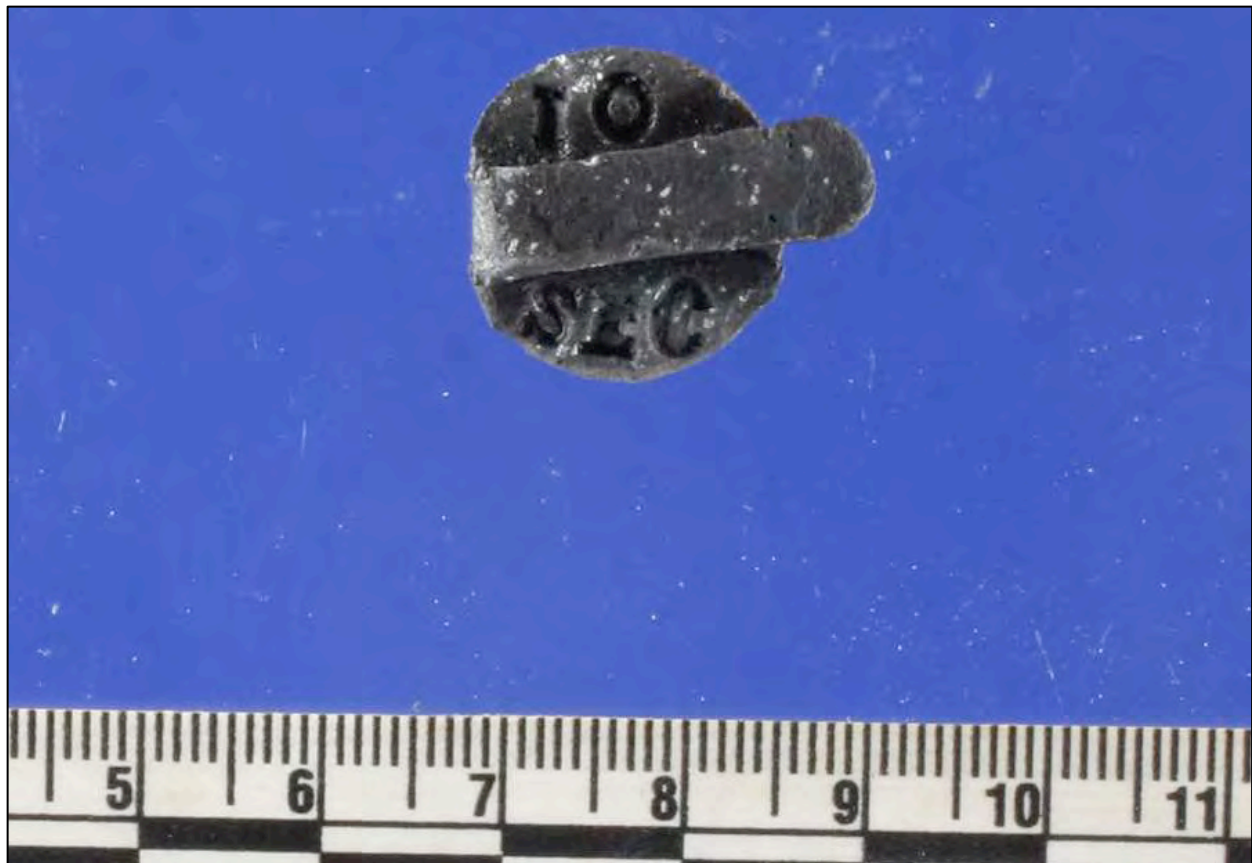
Figure 6-398. Lead safety cap in place on the head of an Alger water-cap time delay fuze that retains an intact pull-tab and displays clear “10”/“SEC” time delay markings, Artifact 2357.1.
