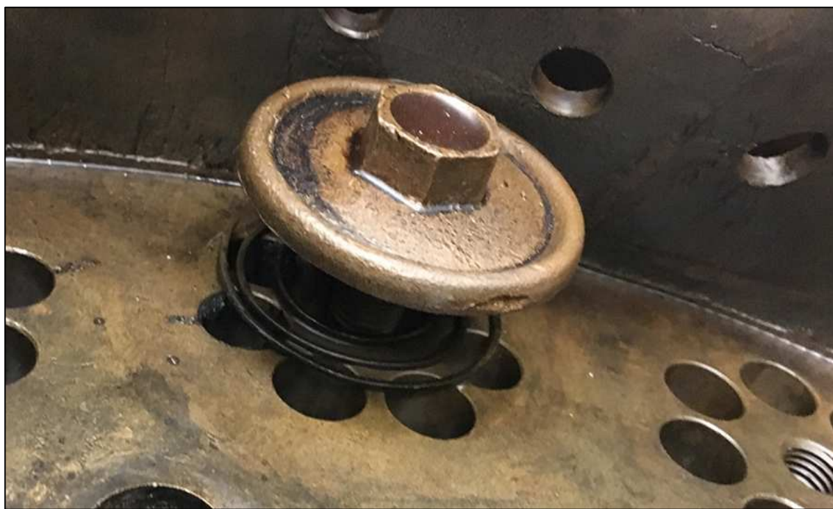
Figure 6-507. Close up of one of the bronze, spring-loaded valves of Artifact 1861.13 put in place after conservation as a demonstration; rubber gasket has been removed.
