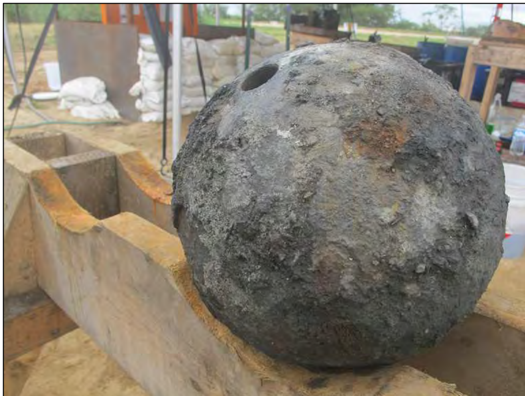
Figure 6-46. Inerted Dahlgren shell with hole drilled for removal of all contents (courtesy of the U.S. Army Corps of Engineers–Savannah District).
