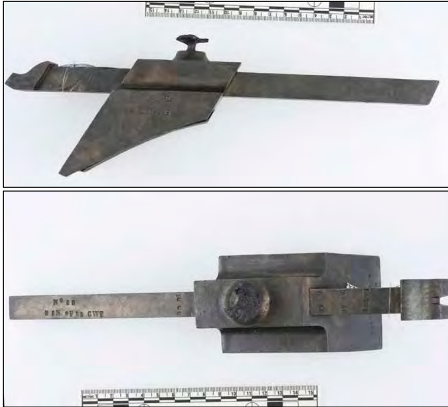
Figure 6-315. Artifact 1892.3 – Top and Side View – Width of “box” 2.4 in. (6.1 cm), Diameter of screw hole: 0.2 in. (0.5 cm), Width of tangent scale: 0.6 in. (1.5 cm), Length of tangent scale: 10.5 in. (26.7 cm). Typical tangent sight. Stamps on scale read: NO 58, 8 IN. OF 55 CWT. Lowest graduation on scale is 260. Largest graduation on scale in 1860. Screw to secure tangent scale still present.
