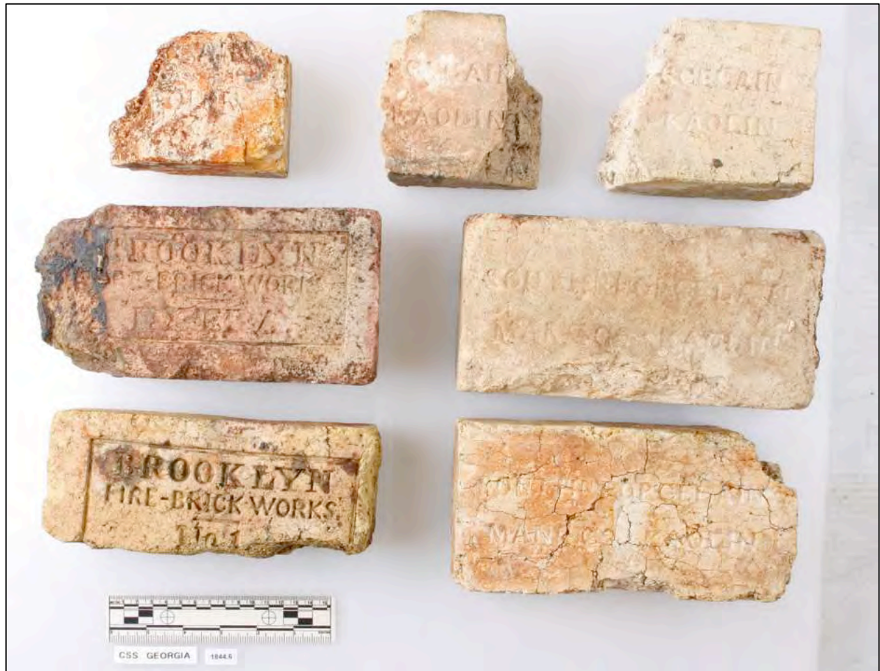
Figure 6-258. Miscellaneous recovered firebricks and brick fragments from the CSS Georgia depicting multiple brands and styles. Artifact 1844.6 from Unit 6-E, the presence of both Brooklyn Fire-Brick Works firebrick and Southern Porcelain Manufacturing Company firebrick from the same provenience as numerous boiler fragments indicates that both were associated with the boiler.
