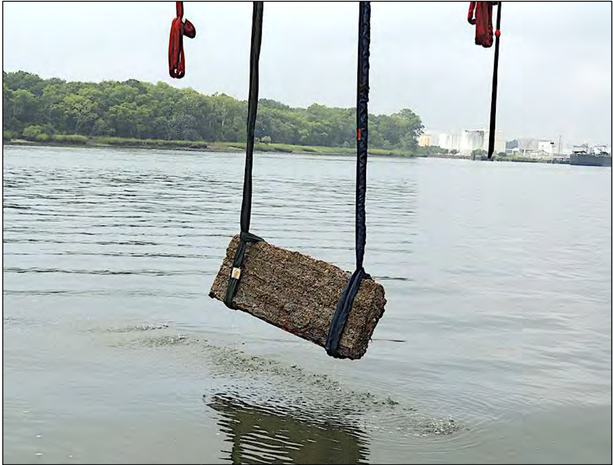
Figure 6-85. Small (No. 3) section recovered from the West Casemate. At first thought to be the bottom of a gunport because of its squared-off top, it would be found that there was a line of fasteners at 8 feet, resulting in many pieces having similar clean breaks at the this 8-foot mark.
