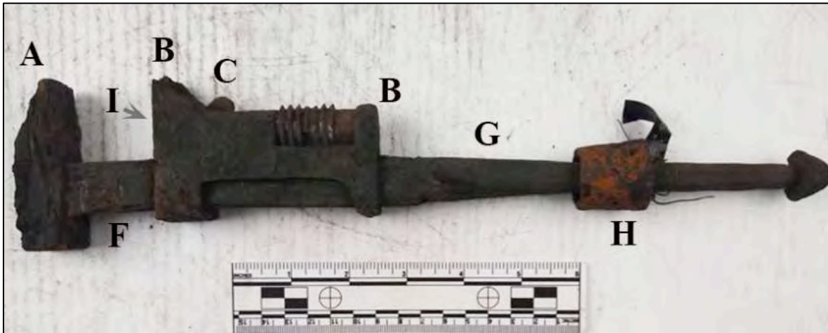
Figure 6-242. Artifact 1879.19, adjustable wrench, parts as follows: (a) upper/fixed jaw, (b) lower/movable jaw assembly, (c) “projection” to engage auxiliary jaw, (d) screw, (e) thumb piece, (f) bar, (g) rod, (h) ferrule, and (i) auxiliary jaw/gripper (obscured in this photo). Labels follow Hyde (1885a; 1885b), while “ferrule” and “rod” are applied from typical definitions of these terms (courtesy of CRL Texas A&M University).
