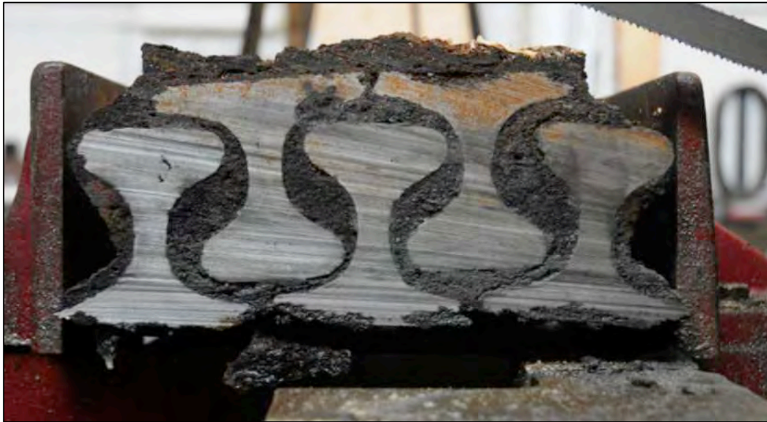
Figure 6-519. Cross section of cut rails for integrity testing showing how the rails were interlocked in two layers, forming a solid flat surface on both sides. Material between rails may be iron fillings as noted above. All rails are shaped alike.
