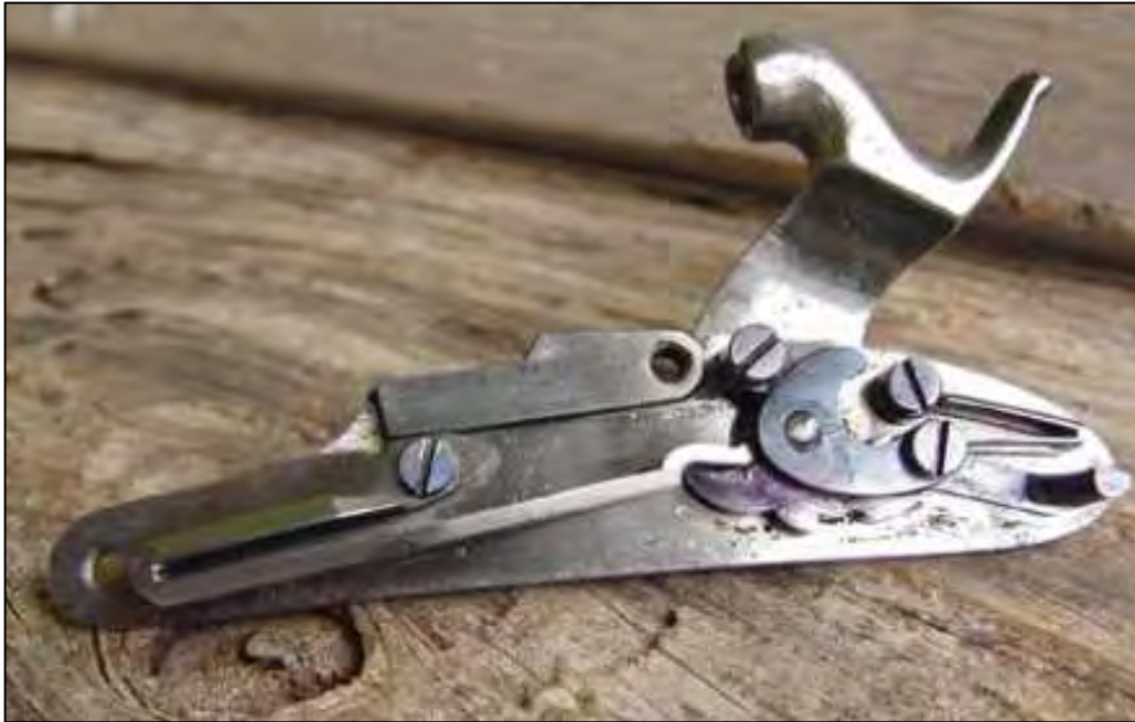
Figure 6-247. Internal view of lock plate from working 1842 percussion pistol (image courtesy of Guns Magazine ).
