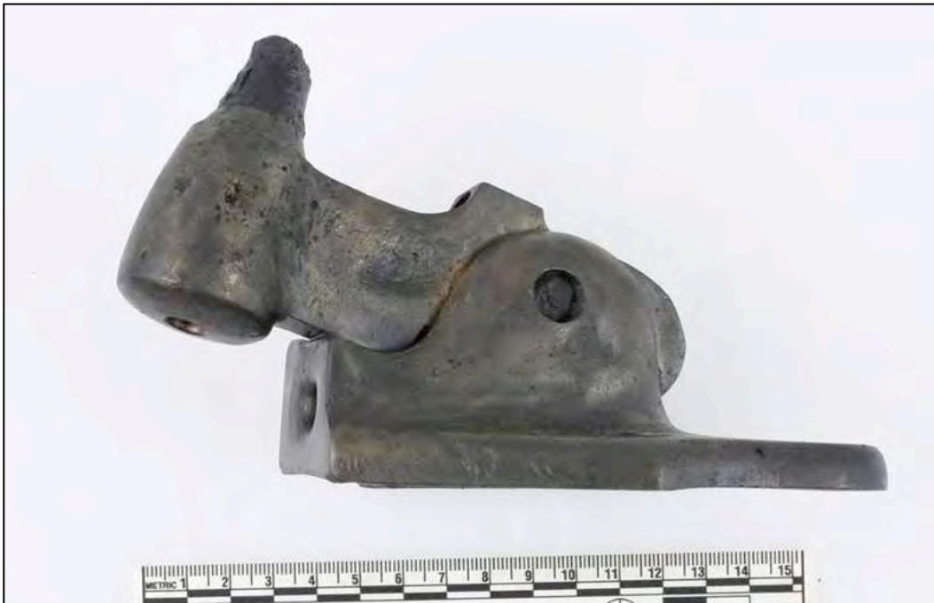
Figure 6-334. Artifact 2012.1 - Lock measurements: L. of shaft: 3.5 in. (8.9 cm), Diameter of “hammerhead”: 1.3 in. (3.3 cm), Diameter of “hammerhead” perforation: 0.4 in. (1.0 cm), L. of iron “nipple”: 0.8 in. (2.0 cm), Diameter of iron “nipple”: 0.7 in. (1.8 cm). A stamp on the top surface of the shaft is not legible due to damage. Perforated “hammerhead.” Base measurements: L.: 5.2 in. (13.2 cm), W.: 3.0 in. (7.6 cm). Base stamp reads: 714.
