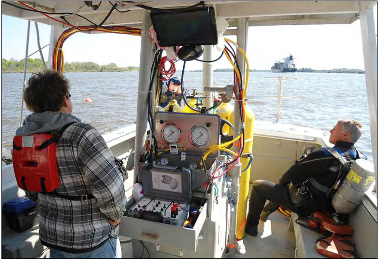
Figure 6-03. Dive station looking aft towards dive tender. Stern mooring ball in the left background. Note redundant yellow air cylinders, dive radio in drawer in front of air manifold, and computer monitor for tracking USBL-equipped diver above. Suited standby diver at right.
