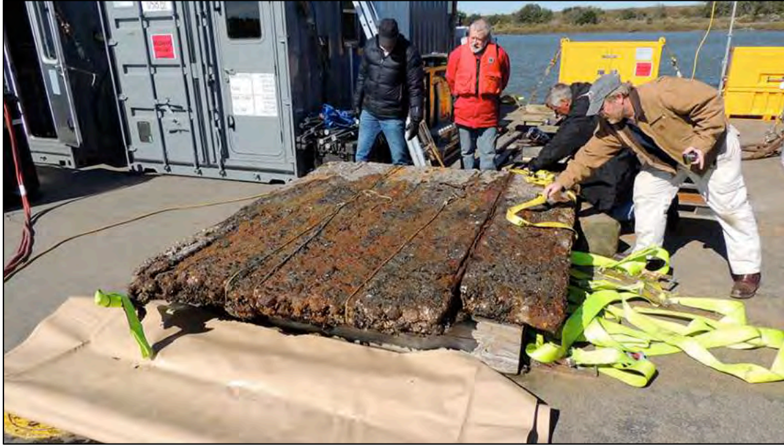
Figure 3-17. Recovery Section with the cradle removed (note ratchet straps). Small section of rail has broken away as evidenced by linear cracked seam.
