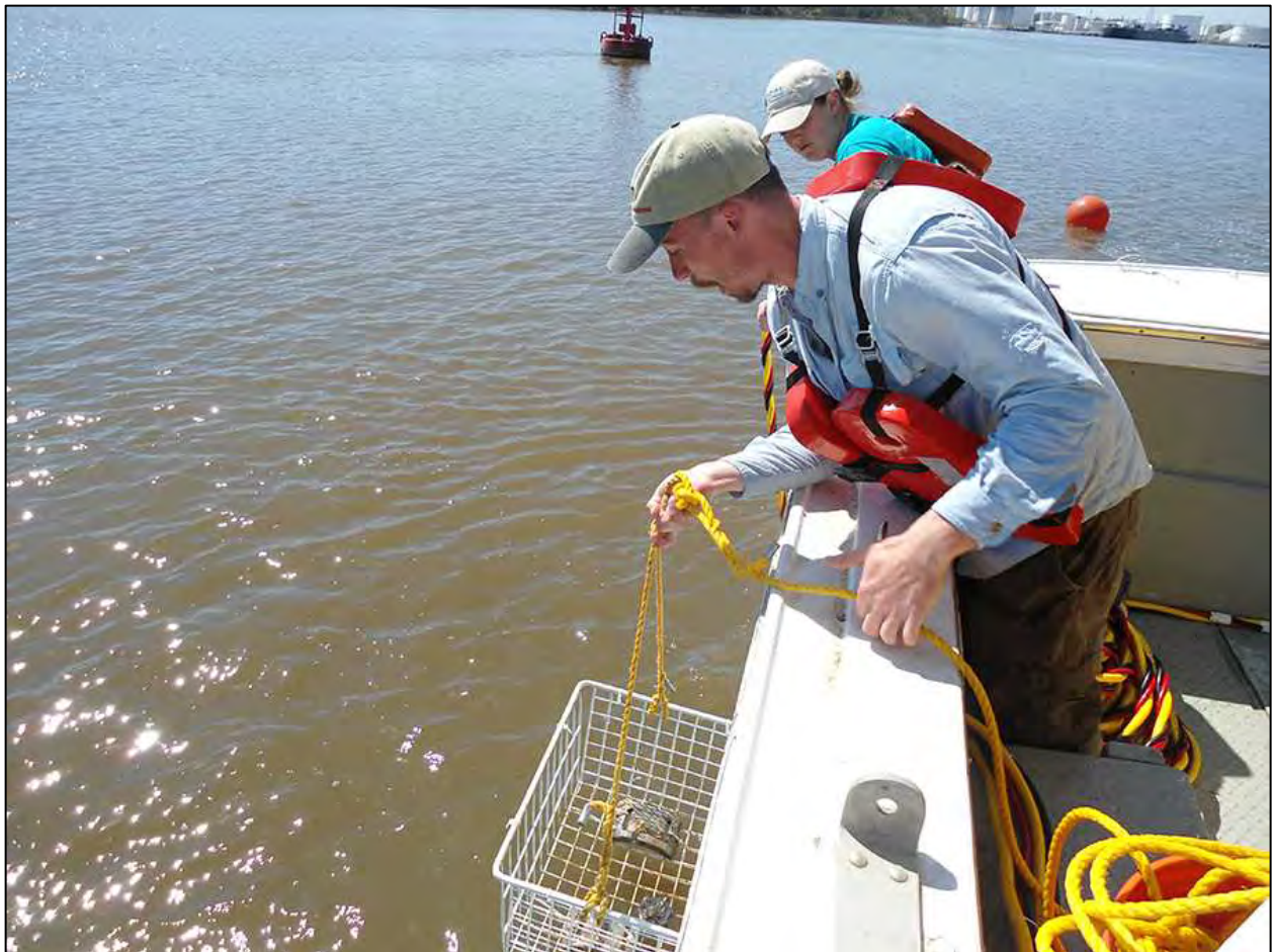
Figure 6-12. Artifact Retrieval Basket being brought to the surface, a very simple yet productive system.
