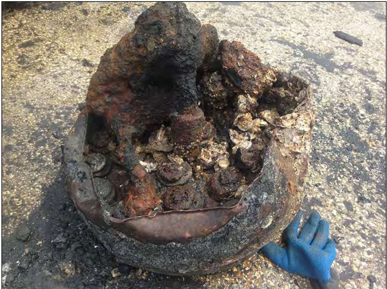
Figure 6-503. Artifact 1861.13, Worthington steam pump component recovered from Unit 5-F. Note the valves and their black circular rubber gaskets, all surrounded by a copper housing.
