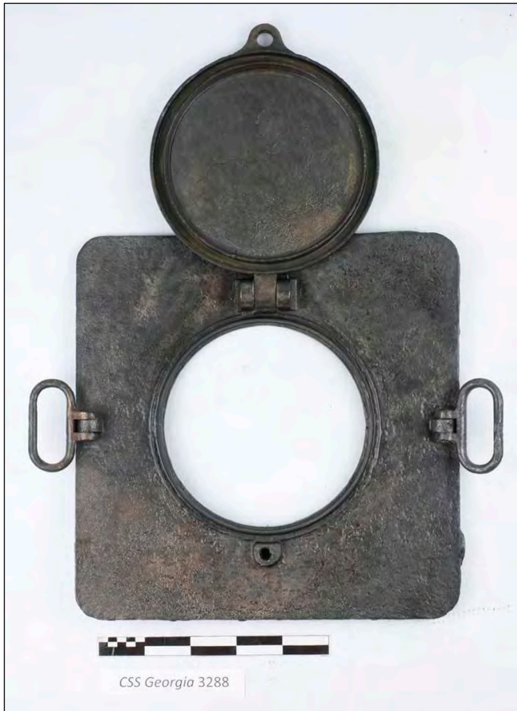
Figure 6-416. Powder tank top showing the handles and the circular opening and the still extant, hinged lid. Note the rubber-gasket lined channel on the lid that seats onto and seals over the raised lip around the circular opening.
