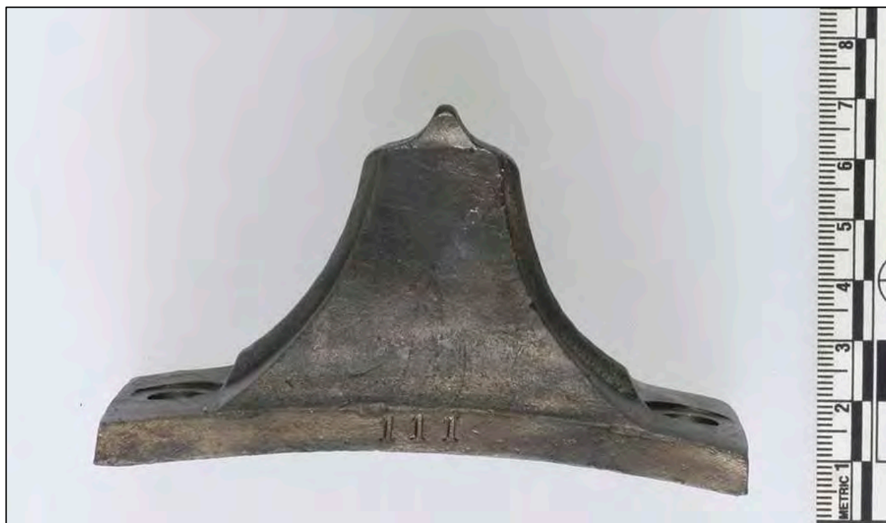
Figure 6-326. Artifact 1856.14 (2 of 2) - Height: 2.0 in. (5.1 cm), W. of base: 1.7 in. (4.3 cm), L. of base: 3.9 in. (9.9 cm). Typical dispart sight. Stamp on base reads: 111.
