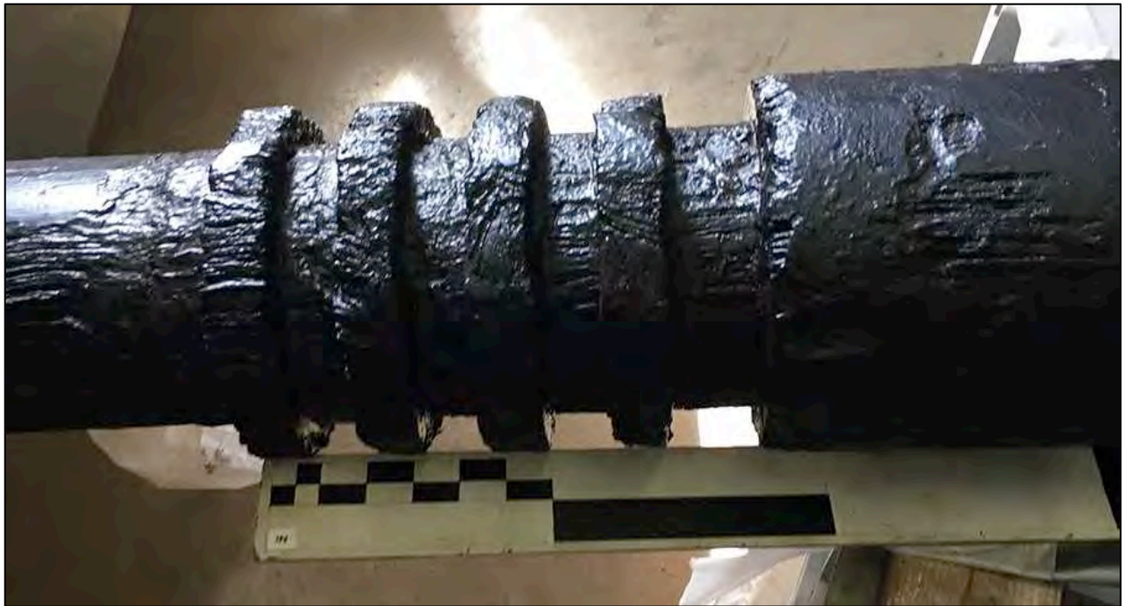
Figure 6-483. Four collars near the end of the propeller shaft that served a thrust bearing.
