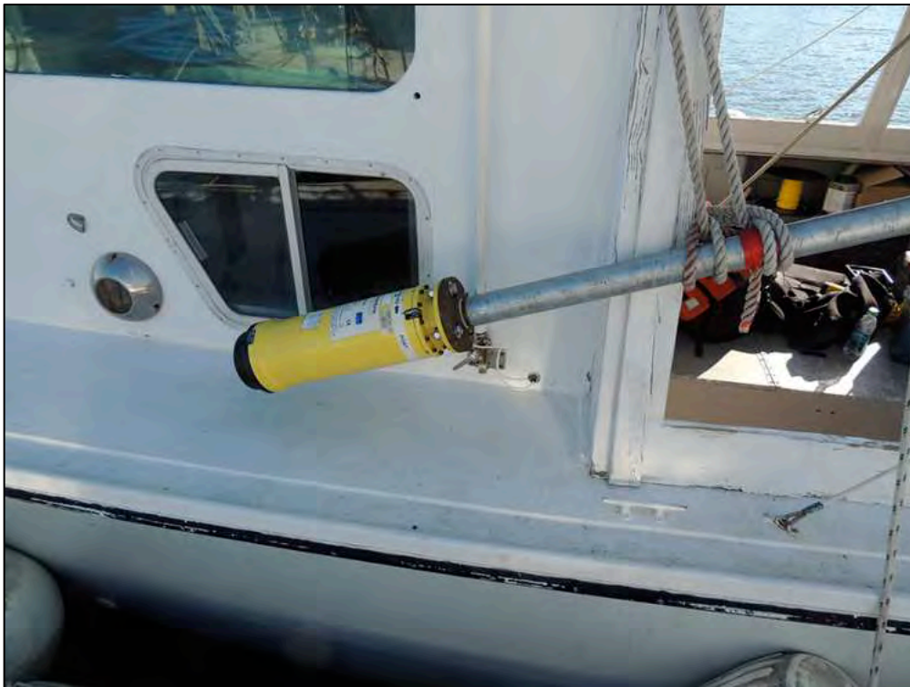
Figure 6-05. Yellow Sonardyne Scout Pro USBL system vessel-mounted receiver lashed amidships during transit to and from the site. Once the vessel was moored up, the receiver would be lowered into the water until vertical (see Figure 6-01).
