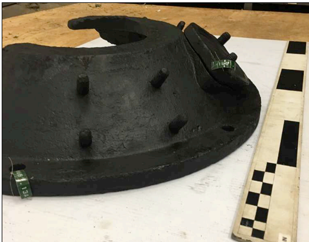
Figure 6-508. Artifact 1861.13, Worthington direct-acting steam pump cast iron cover. This attached to the base of the bronze valve plate above and is thought to represent the bottom of the pump.
