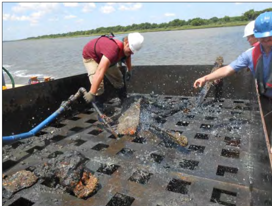
Figure 12. Initial processing of a Clamshell grab. Screen was difficult to access and affected processing efficiency.
