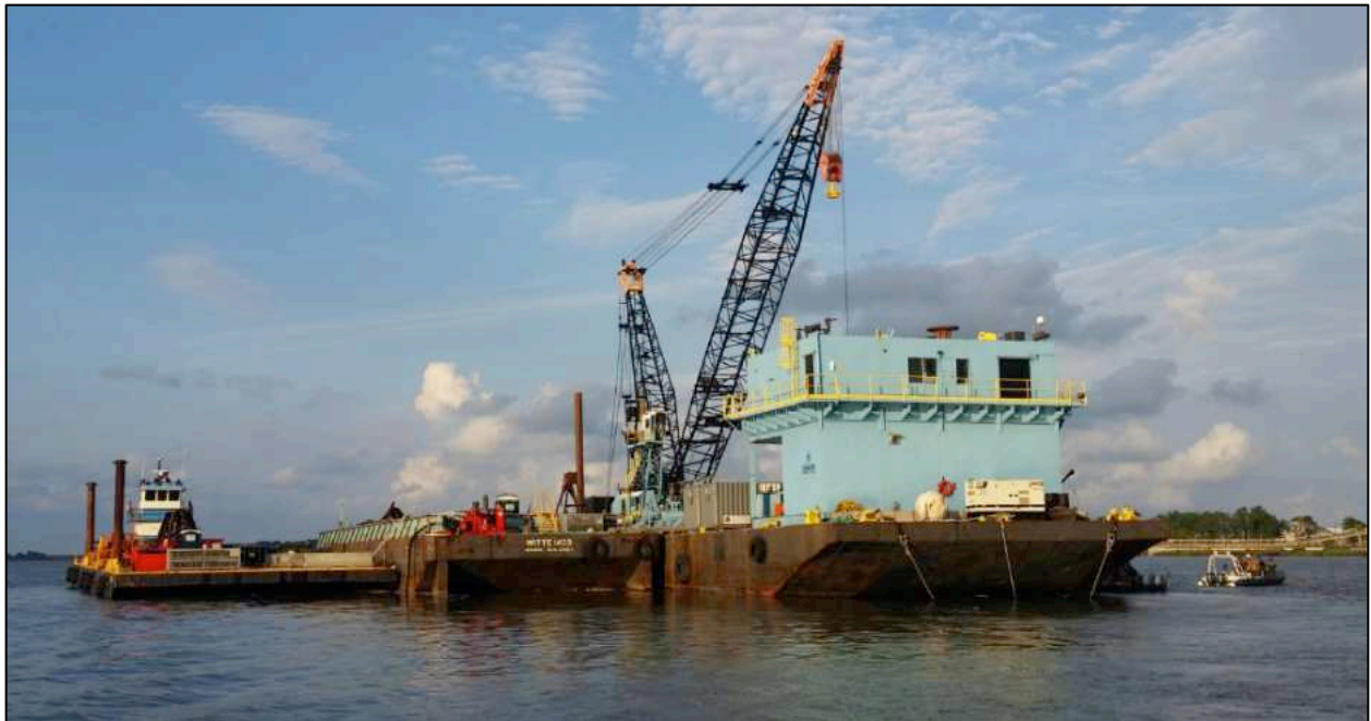
Figure 6-86. The work platforms for the 2017 Operation recovery effort consisted of the Farrell 256 Crane and Dive Barge (right), the Witte 1403 Hopper Barge for casemate storage (center), and a smaller material spud barge for mechanized recovery and screening (right).
