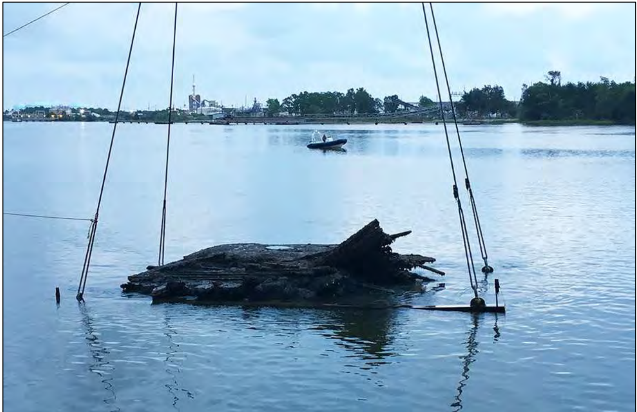
Figure 6-89. East Casemate breaking the surface during recovery. At this point it was found to weigh 23.5 tons (43.5 tons with the lift frame).
