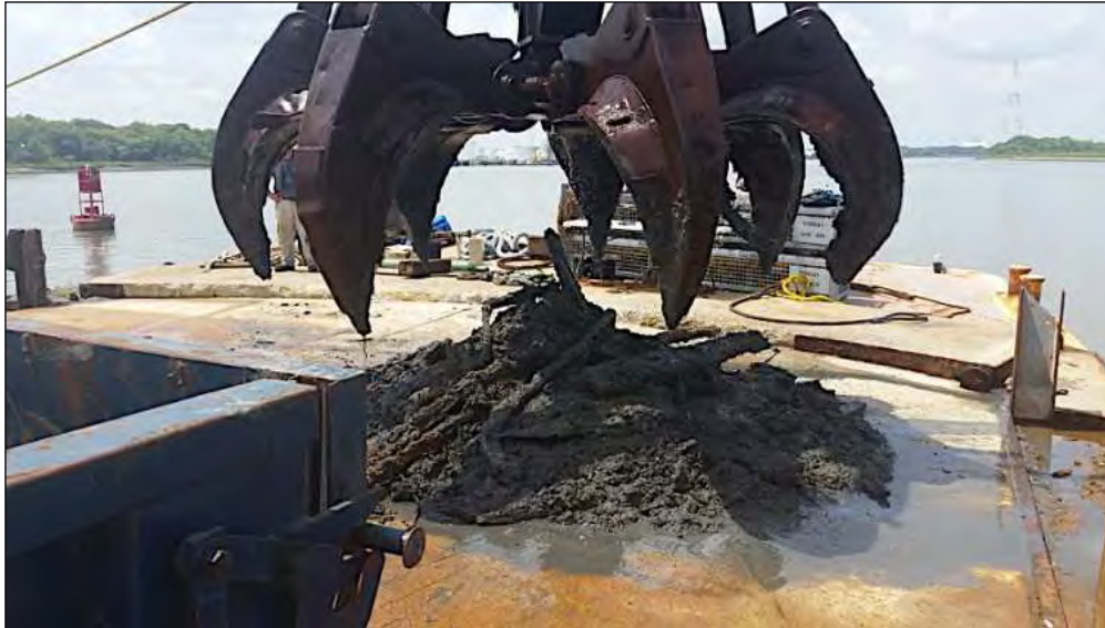
Figure 6-104. 14-ton, seven-finger grapple depositing initial test on deck. The sediment matrix was carefully hosed off the barge to the right and away from wreck site. The first six grapple tests were easily sorted and washed with no loss of material, even with the absence of a screen.
