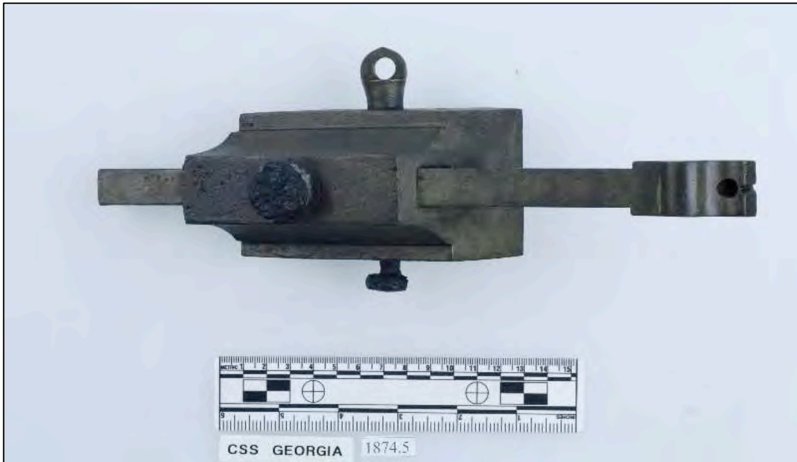
Figure 6-319. Artifact 1874.5 - W. of “box”: 2.4 in. (6.1 cm), W. of tangent scale: 0.6 in. (1.5 cm), L. of tangent scale: 10.9 in. (27.7 cm). Has a slightly different appearance from the other tangent sights. The head of the scale is perforated with a small hole. Graduations are in degrees. Stamp on scale reads: NO. 3 OF 66- and then it cuts off. Stamp on “box” reads: NO 3 OF 6600.
