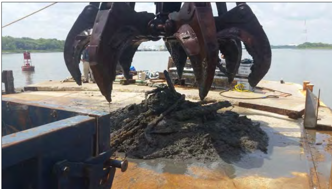
Figure 8. Raising of a Grapple. Grapple G1 surprisingly collected more sediment as well as cultural material than clamshell. Material hosed off of barge to the right and away from wreck site. Grapple sample was easily sorted and washed with no loss of material even with the absence of a screen.
