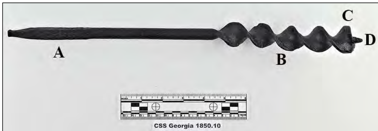
Figure 6-218. Artifact 1850.10. Auger parts as follows: (a) shank, (b) spiral, (c) cutting edge, and (d) leading screw (courtesy of CRL Texas A&M University). Labels follow terminology in Blackburn (1998:316) and Mercer (2000:200).
