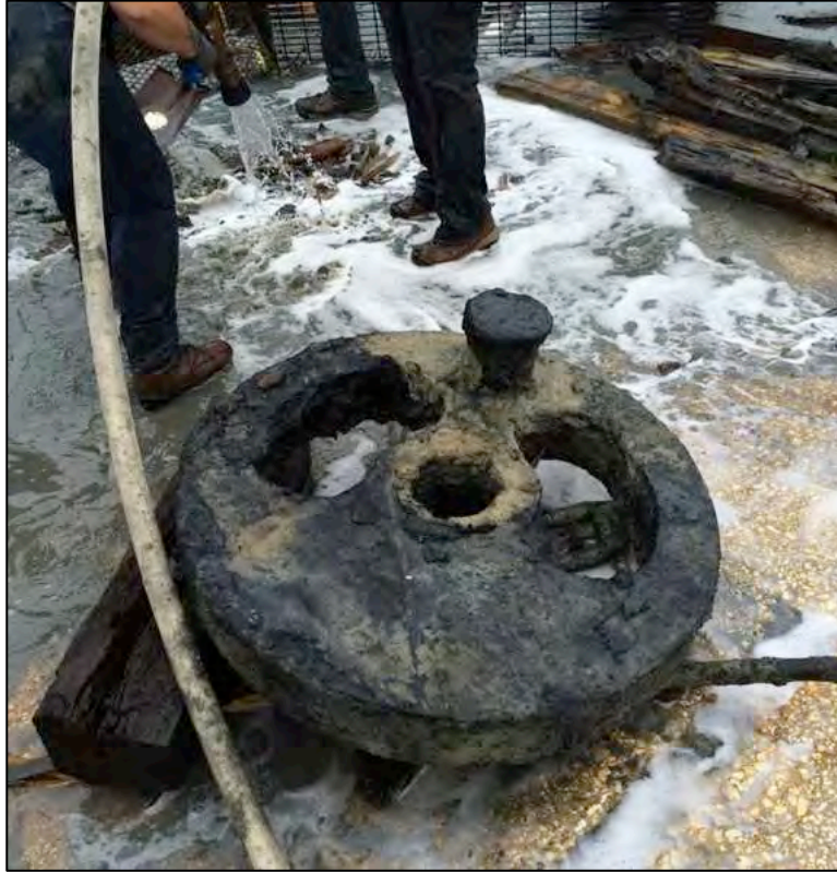
Figure 6-489. Shown at the time of Mechanized Recovery, counterbalance flywheel that was connected to the end one of the vessel's two propeller shafts, and turned by a crank connected to one of the two steam cylinders, which would then turn the propeller. The crank attachment is the projection at top. Artifact 1899.17 recovered from Unit 6-C.
