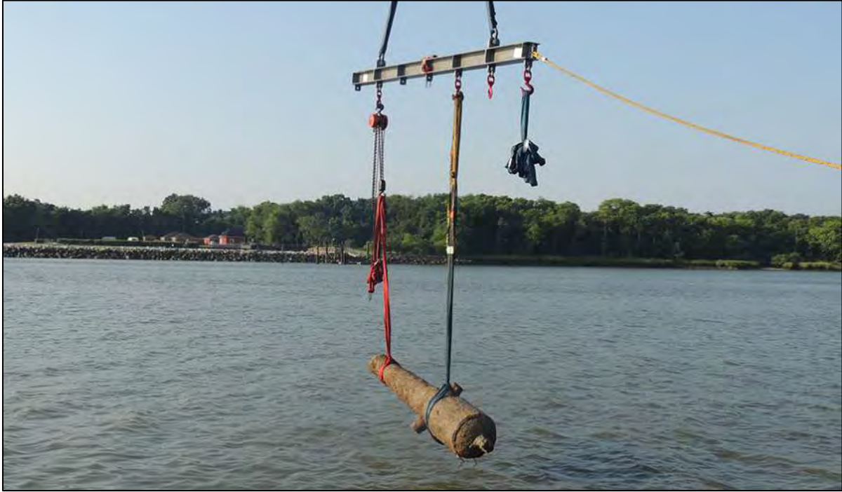
Figure 6-36. Method of rigging cannon for lifting. Cannon 2 is shown being lifted, one “roundsling” placed just aft of the muzzle, the other just aft of the trunnions. Note the USBL transponder on the top center of the beam for positioning over the cannon for easy diver location.
