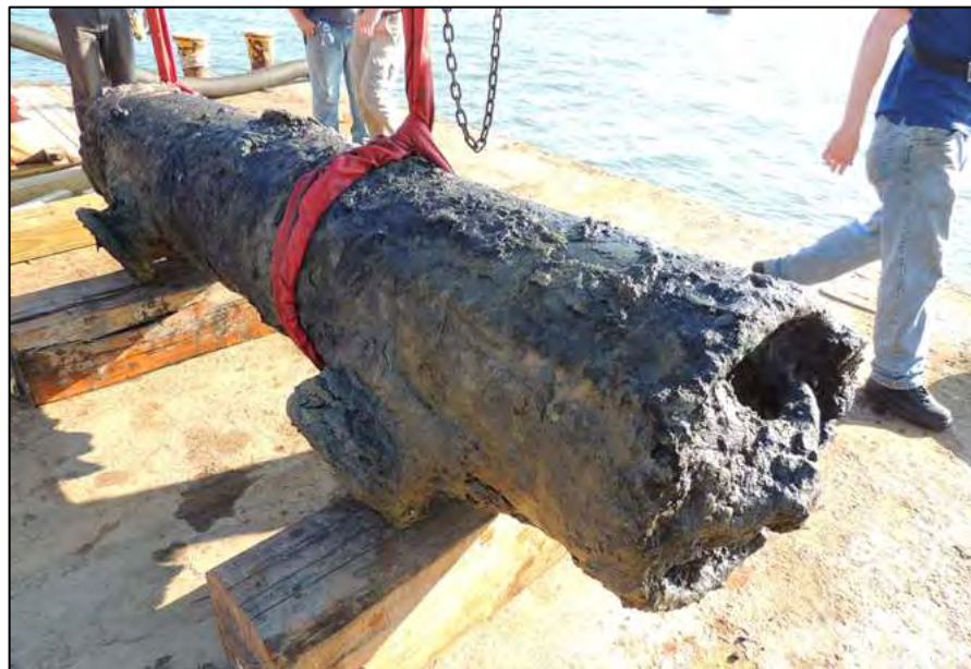
Figure 6-50. First identified as a condenser, it is possible that the riveted cylinder represents a mud drum.
