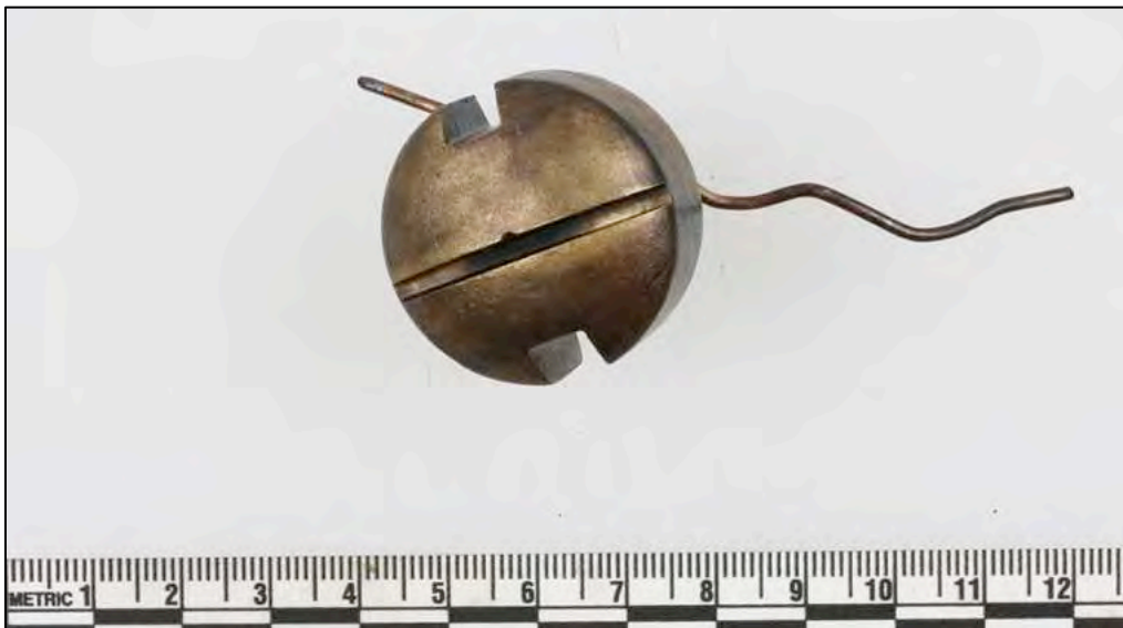
Figure 6-393. Top view of the Archer fuze clearly showing the off-center position of the safety pin or wire, Artifact NP5. Also note facets for screwdriver or naval fuze wrench.
