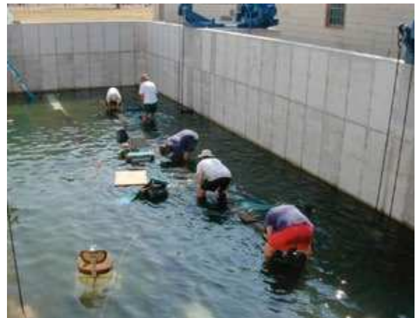
Using the water to reduce the weight, the staff turn the keel over to clean the other side
