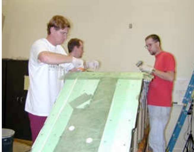
Preparing the vacuum bag to make the frame plate.
