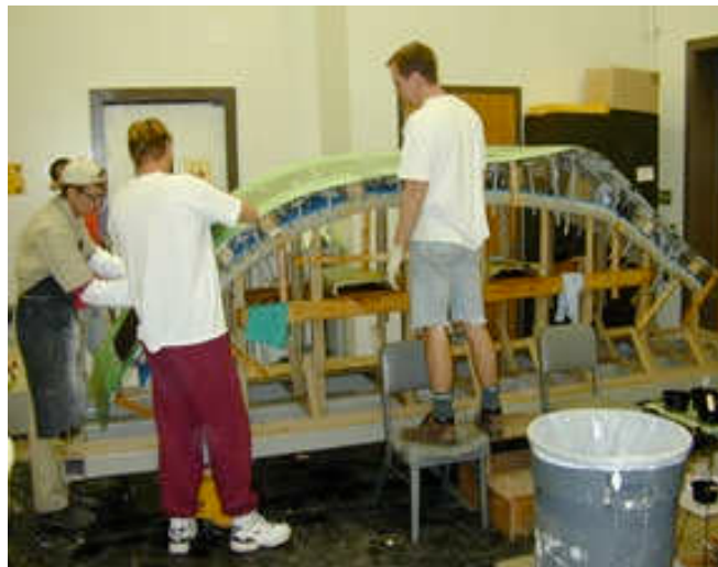
A frame set is positioned on the molding frame so that a carbon fiberglass composite plate can be cast.
