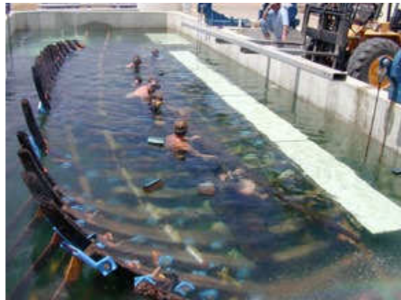
Lab assistants use the weight of the water to displace the weight of the keelson so that it can be placed in position and the frames more carefully aligned.
