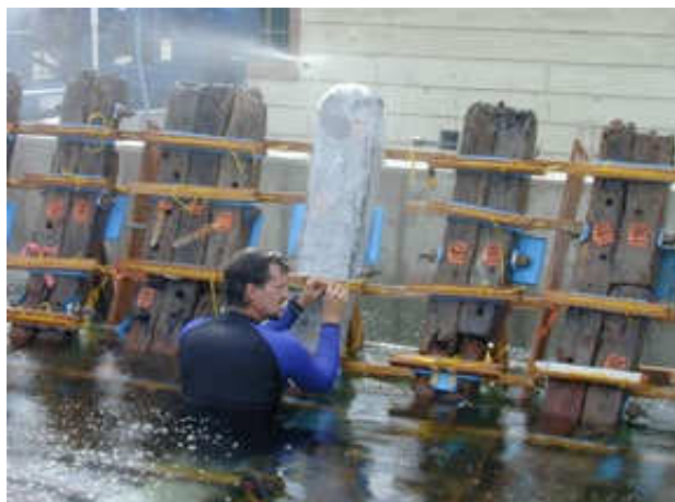
Taras Pevny and Peter Fix position a frame set back into sequence after creating a laminate. This process is required for each frame set. Note the weather is much colder, requiring the workers to wear wet suits and hats.
