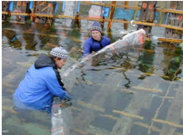
Preparing the vacuum bag to make the frame plate.
