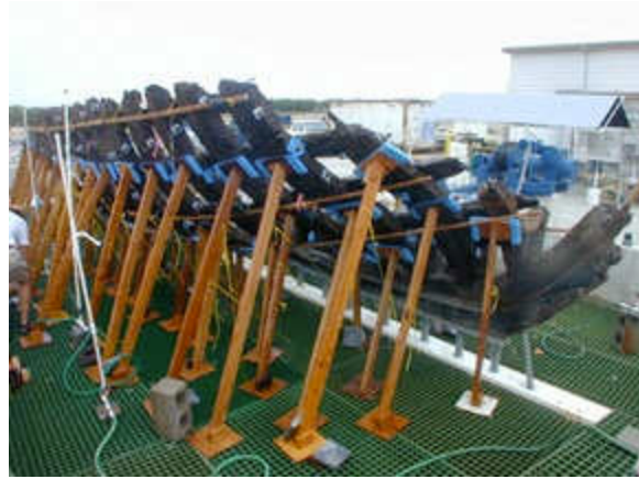
Note the supports being used to support the frame sets. Once the support plates are positioned on each frame set, the ship will be able to stand with minimal external supports while on display.
