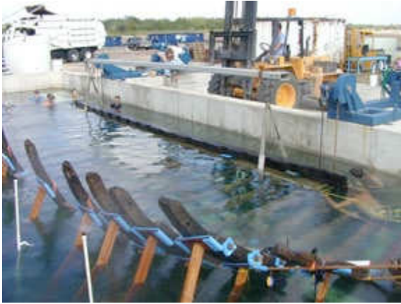
Using a large forklift and spanner bar to place the keelson in the vat.
