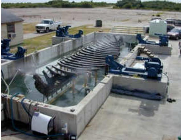
Placing the frames on the keel floors.
