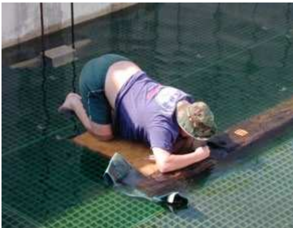
Sometimes it's necessary to get really close to your work to get all of the crud out of the holes and the junctures in the keel.
