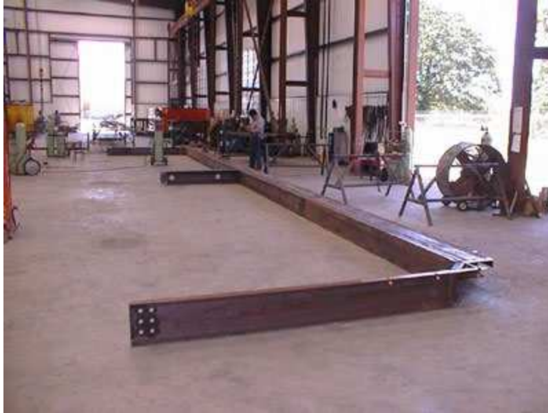
One side of the lifting frame is being welded together in the Dynacon, Inc. shop in Bryan, Texas.
