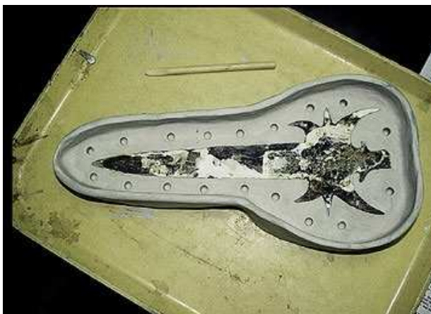
Part metal/metal oxide and part epoxy partisan as removed from the encrustation after filling voids with epoxy
