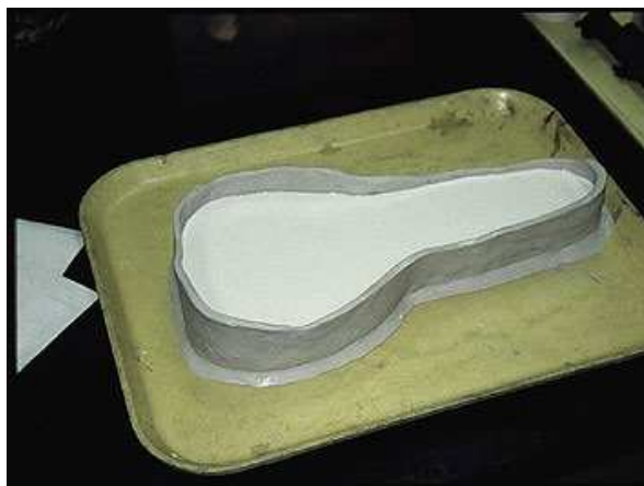
Silicone rubber mold cast with Hysol LE 6329 NA epoxy
