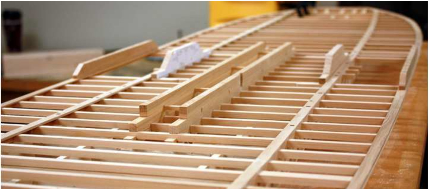
Figure 1: Model of Heroine 's main deck. Most of the main deck structure has survived on the wreck.
