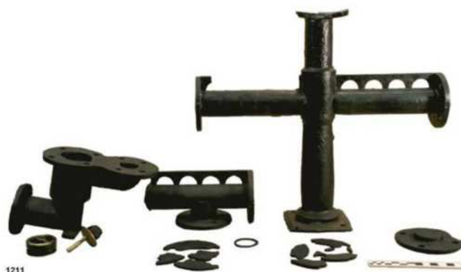
Figure 2: Fragments of two cast iron standpipes and a high-pressure check valve
